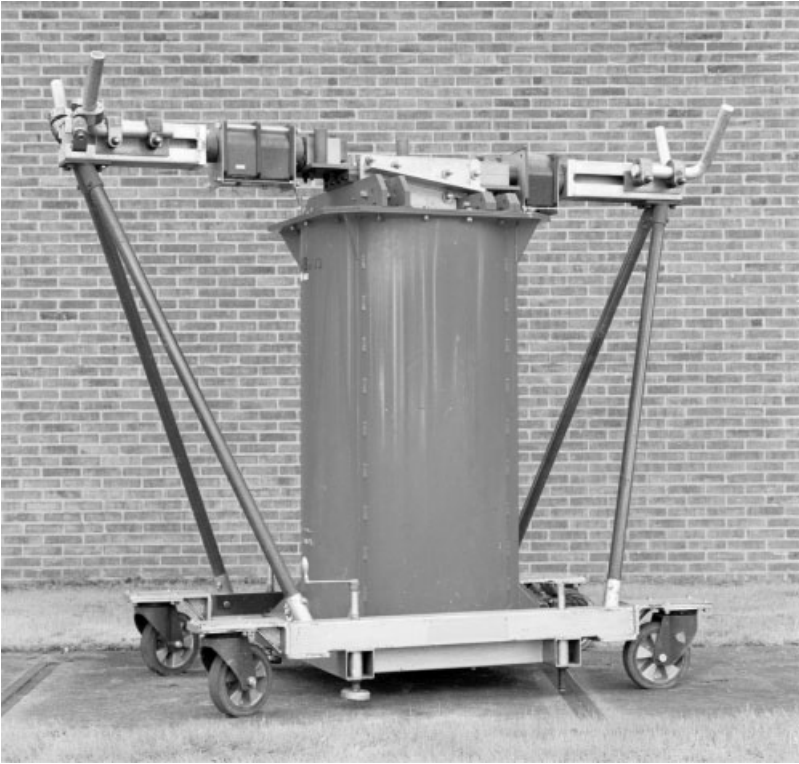
Figure 10.23 Coaxial shunt for measuring currents up to 100 \text{ kA}_{\text{rms}} with a bandwidth of 0–1 MHz (courtesy of KEMA)
