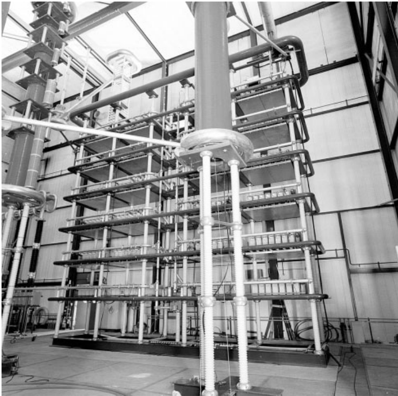
Figure 10.17 Main capacitor bank C_0 and main inductance L_1 of KEMA's synthetic test facility (courtesy of KEMA)
