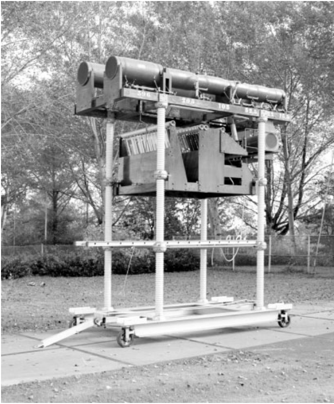
Figure 10.21 Artificial line to be used for short-line fault testing in a parallel current-injection circuit (courtesy of KEMA)
