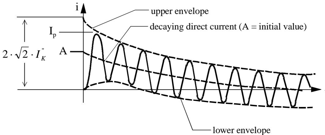
**Figure B-16: Short-circuit close to generator with missing current zeros**
