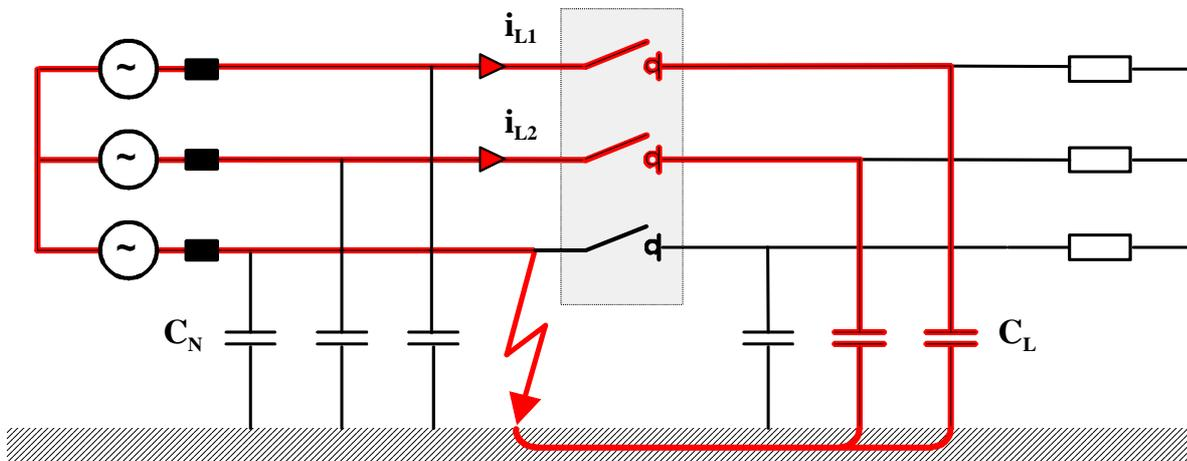
Route of the capacitive load current, e.g. in the healthy phase L2, that must be switched off by the breaker.
