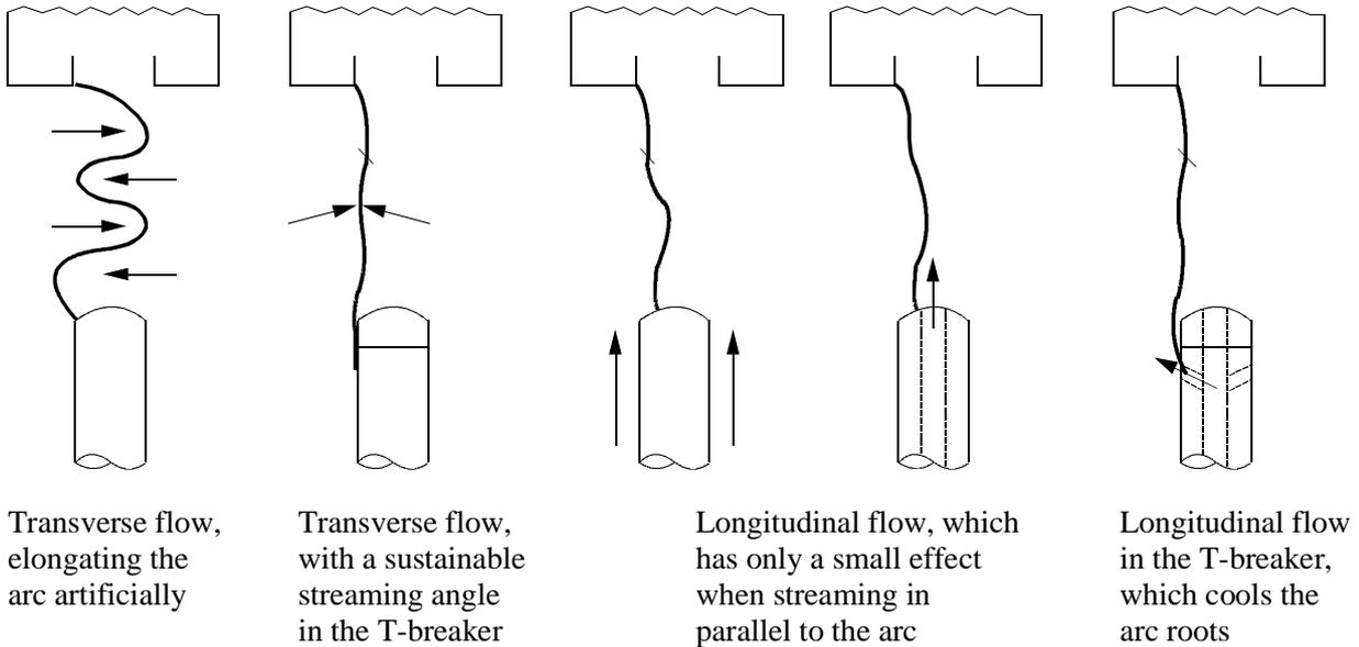
**Figure C-2: Arc-quenching in minimum-oil circuit-breakers**
