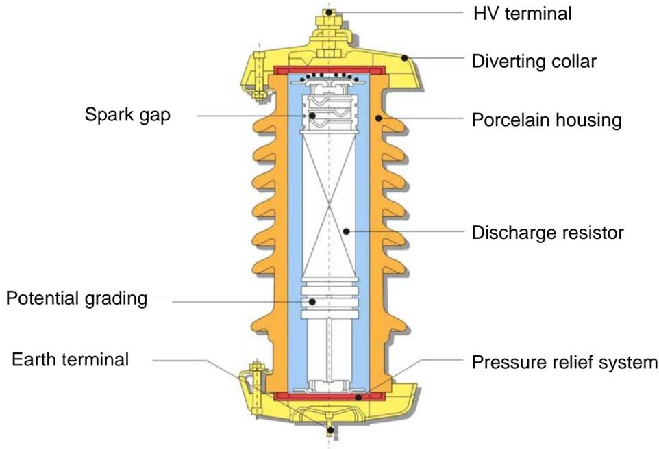
Figure C-26: Surge arrester (example Siemens 3EG type)
