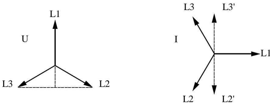
**Figure B-18: Vector diagram of a short-circuit in the system**
