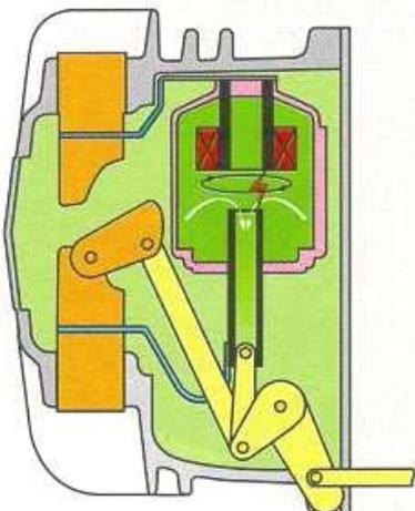
**Figure C-5: Example of a self-extinguishing SF<sub>6</sub> circuit-breaker**
