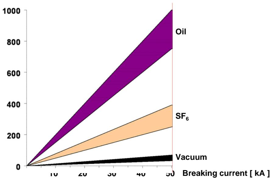
**Figure C-9: Arc energy in different quenching media in the comparison**
