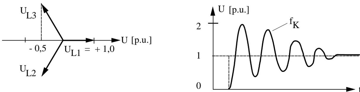
**Figure B-8: Voltages at time  $t_1$  and voltage trace in first pole to close**
