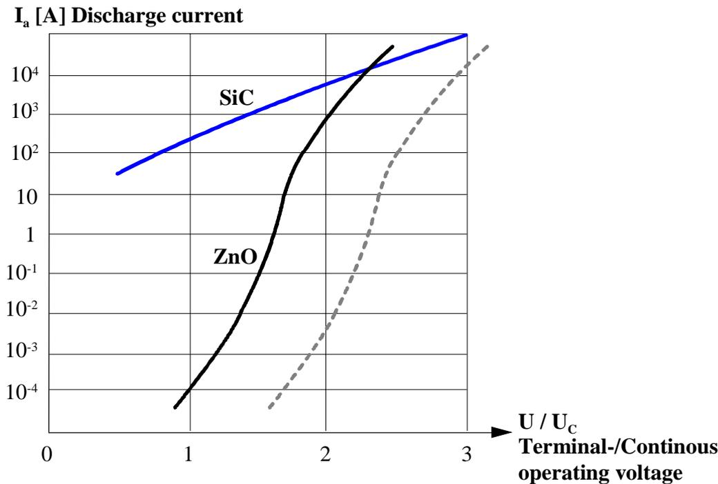
**Figure C-29: Current voltage characteristics of SiC and ZnO**
