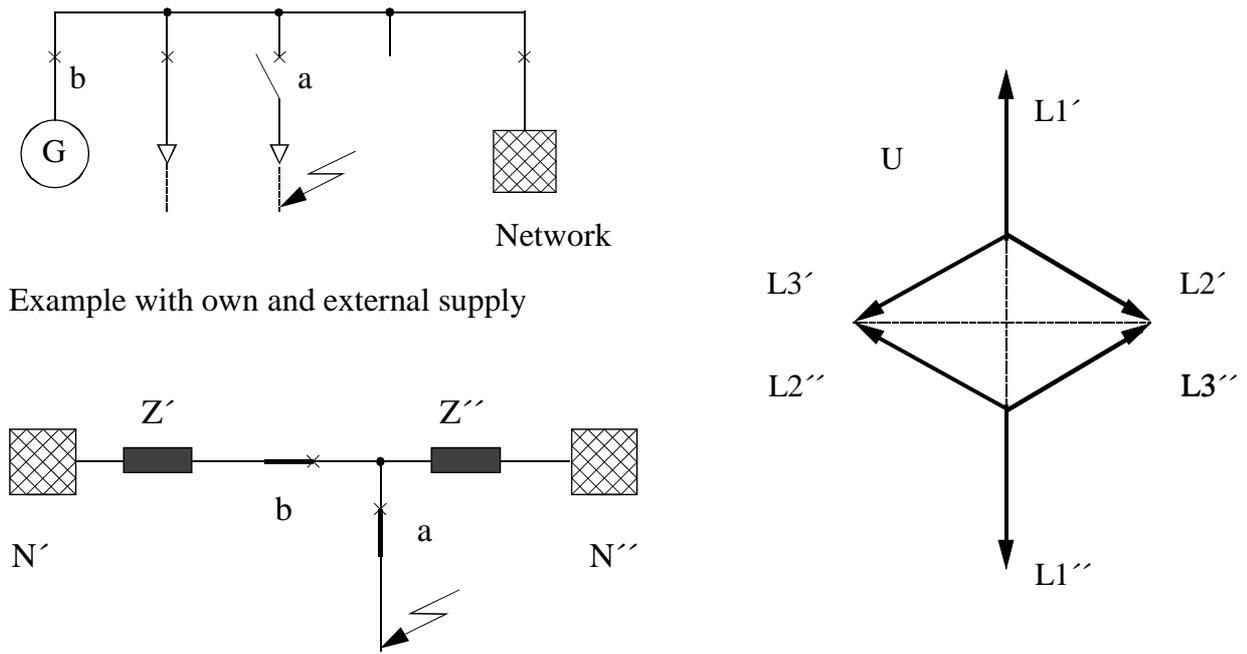
**Figure B-23: Switching off under out-of-phase condition**
