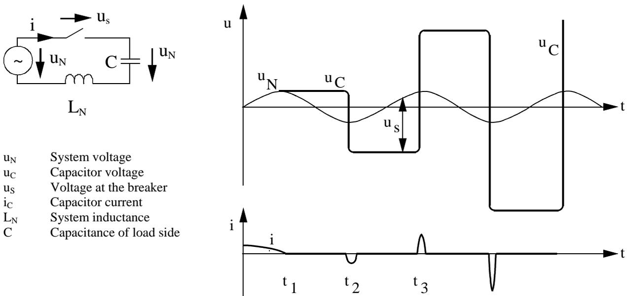
Figure B-11: Restrikes during capacitive switching
