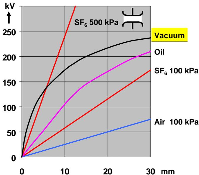
**Figure C-7: Discharge voltages as a function of the contact stroke in different media**
