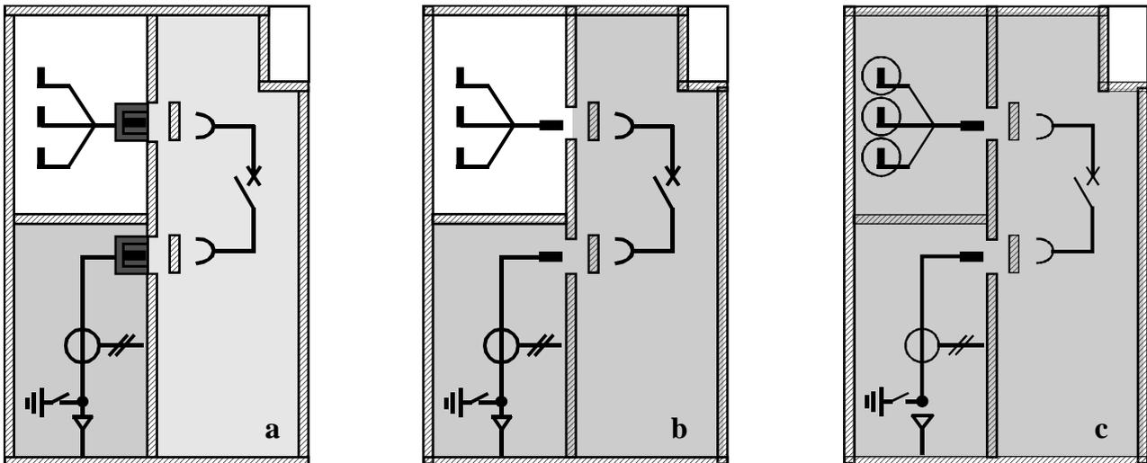
**Figure E-3: Withdrawable or truck-type design with „compartmentalization“**
