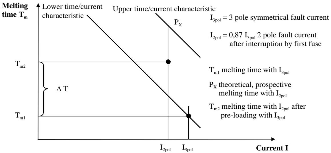
Figure C-23: Melting time of fuse in the region of the transfer current
