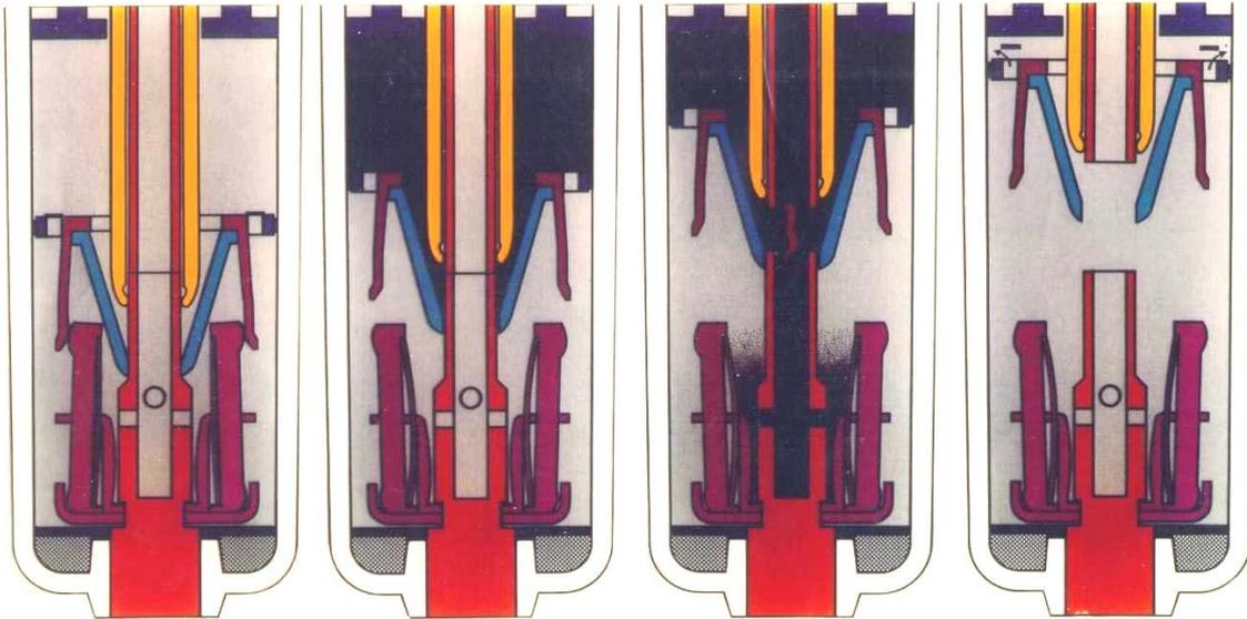
**Figure C-4: Arc-quenching principle of an SF<sub>6</sub>-puffer type circuit-breaker**
