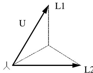
Voltage  $u_N$  in case of earth fault in L3
