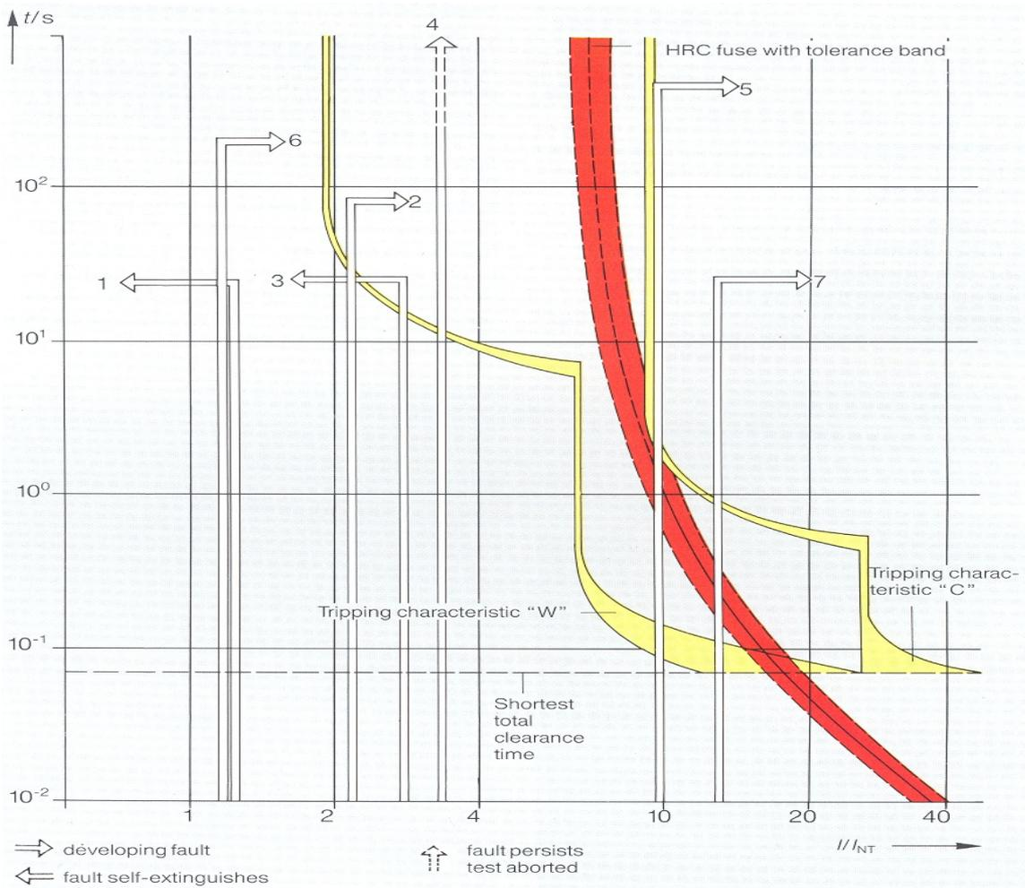
**Figure C-24: Fault currents and tripping characteristics of the protection devices**
