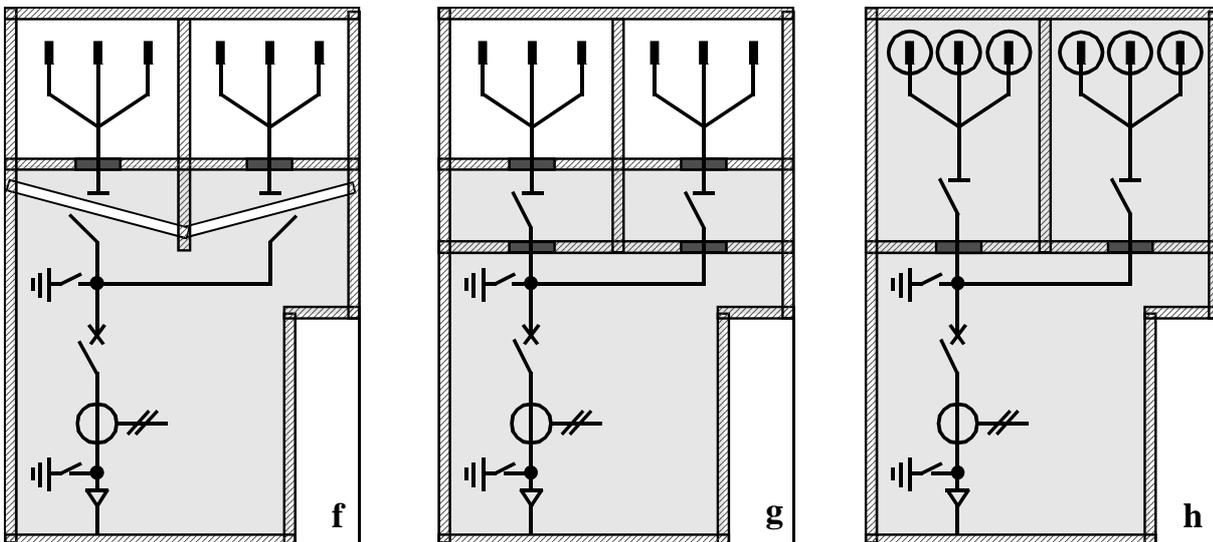
**Figure E-26: Cubicle design double busbar switchgear**
