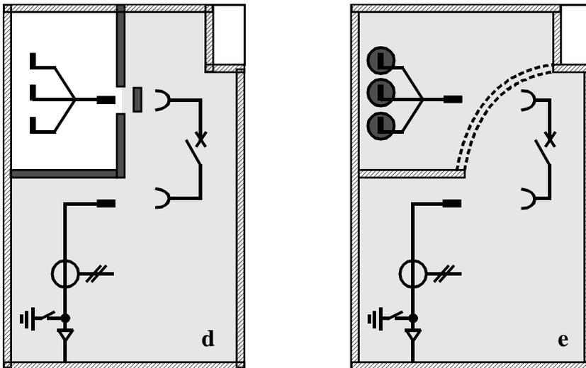
**Figure E-4: Cubicle design with withdrawable or truck-type switching device**
