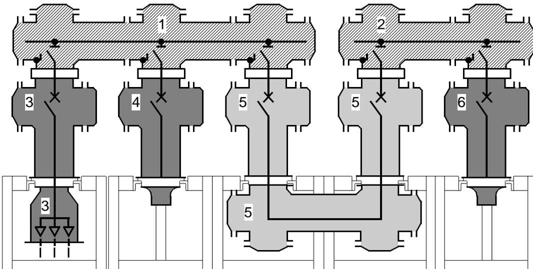
**Figure E-18: Gas compartments of a single-pole encapsulated switchgear cross-section of double busbar (equal numerals = equal gas compartments)**
