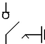
Three-position switch-disconnector and make-proof earthing switch
