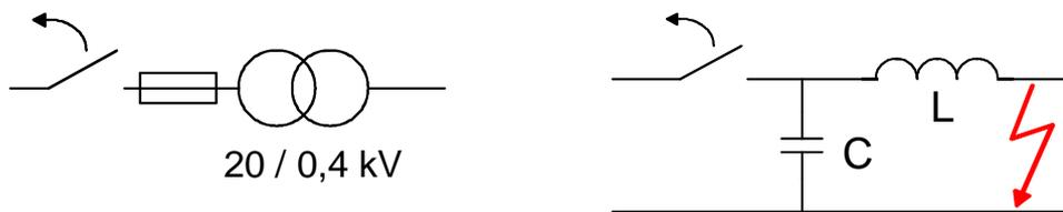
**Figure B-21:** Short-circuit downstream transformer
