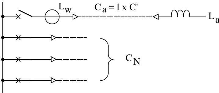
**Figure B-7: Network and load capacitances on closing**
