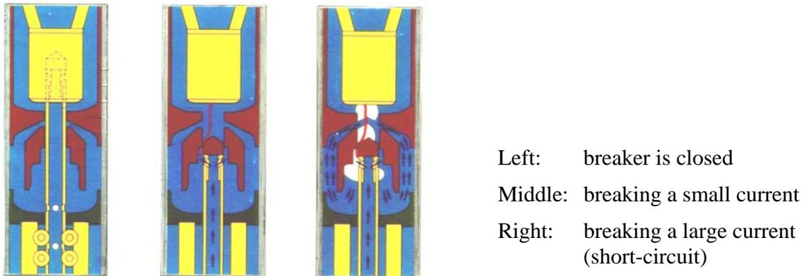
**Figure C-3: Example of a minimum-oil circuit-breaker with combined oil flow**
