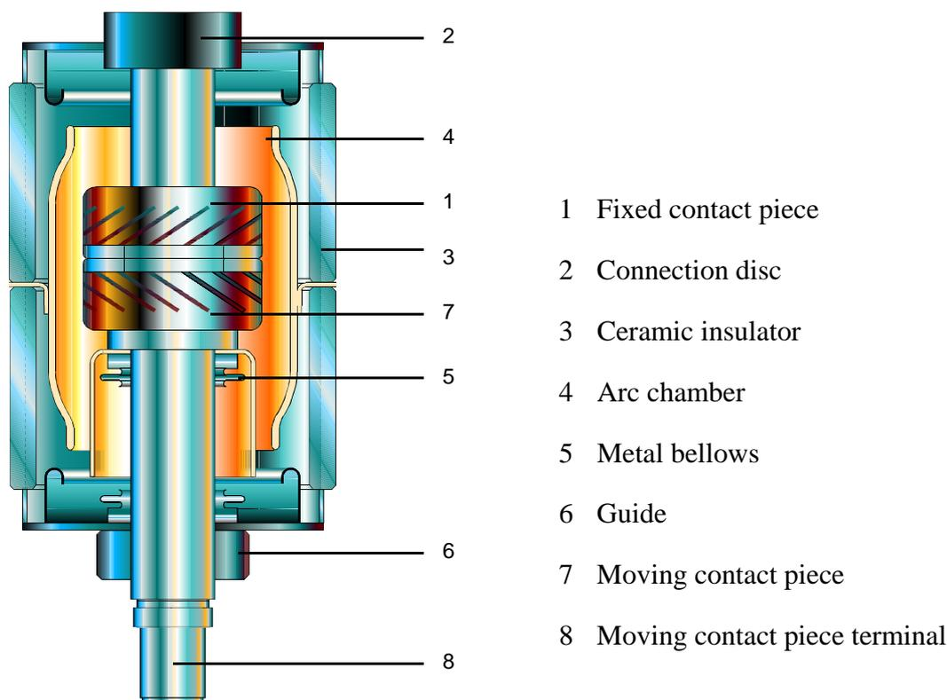
**Figure C-6: Structure of a vacuum interrupter**
