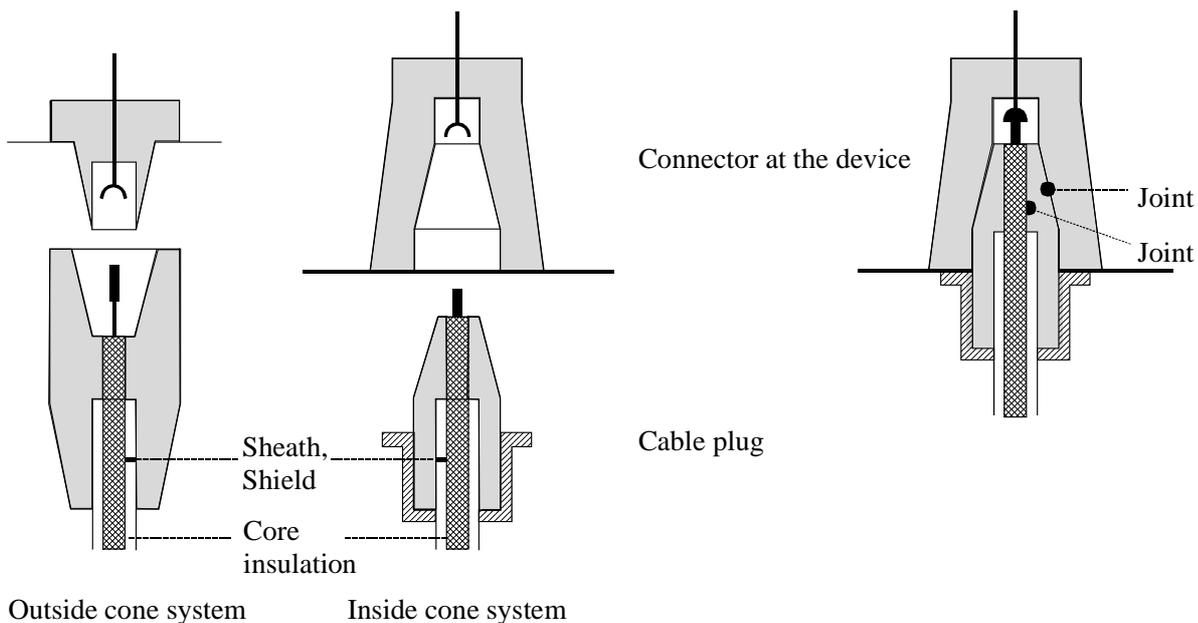
**Figure F-4: Scheme of inside and outside cone system**
