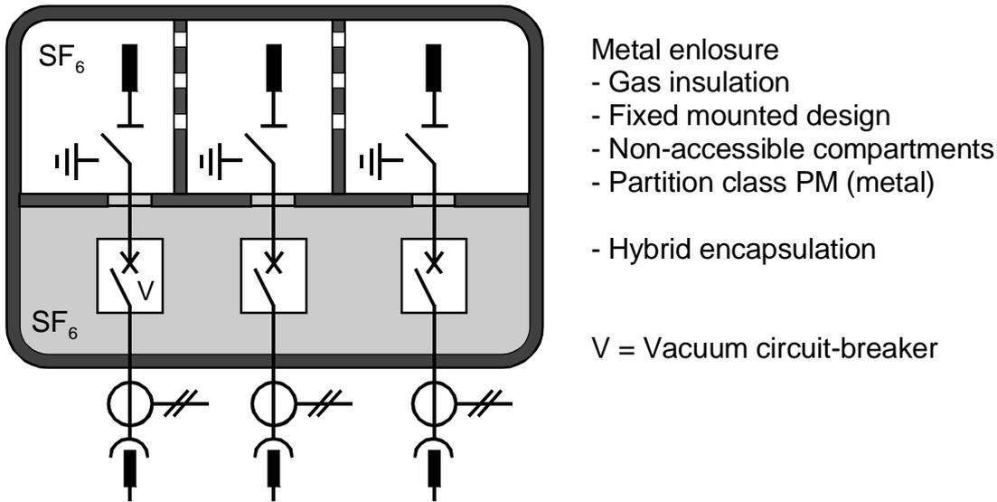
**Figure E-8: GIS design with hybrid encapsulation**
