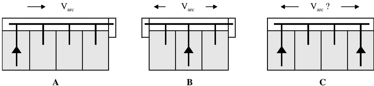
**Figure E-5: Direction of fault arc travel for various locations of incomer**
