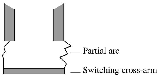
Some of these disadvantages were overcome by the introduction of arc chambers under the oil. The switching characteristics of these designs correspond approximately to those of minimum-oil circuit-breakers with a current-dependent arc-quenching effect.
