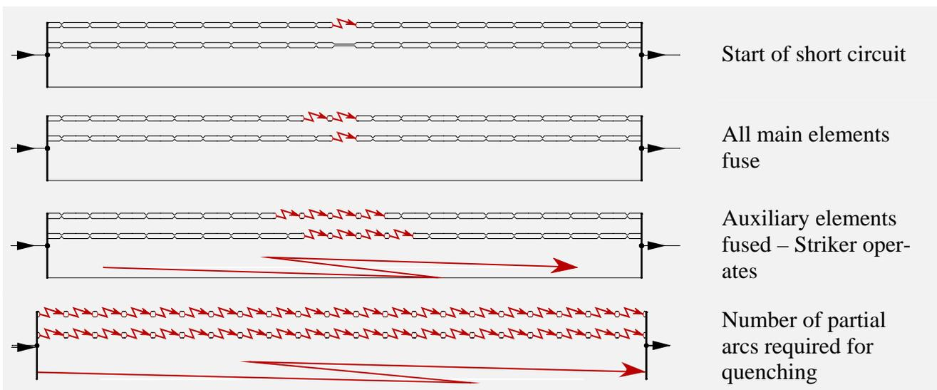
**Figure C-15: Phases of breaking**
