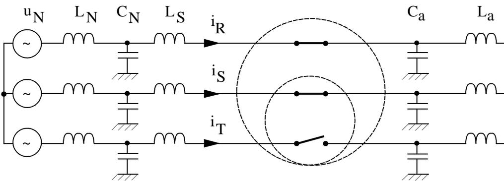
Figure B-5: Coupling to the phases S and R due to multiple reignitions in phase T
