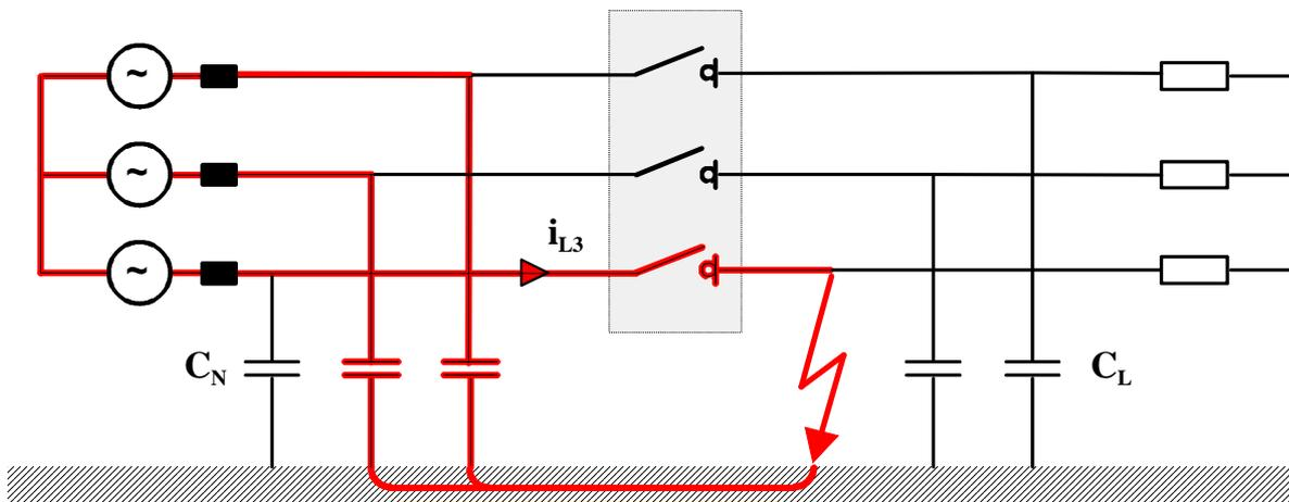
Route of the capacitive load current of the entire galvanically connected system, that must be switched off by pole L3 of the breaker.
