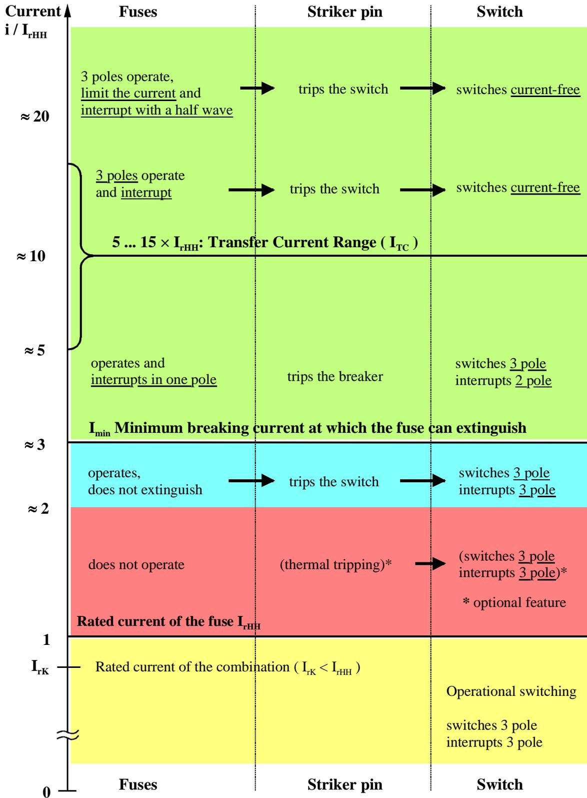
Figure C-21: Interaction between switch and fuses in combination
