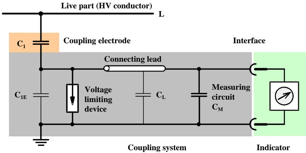
Figure F-8: Scheme of a separable voltage detecting system
