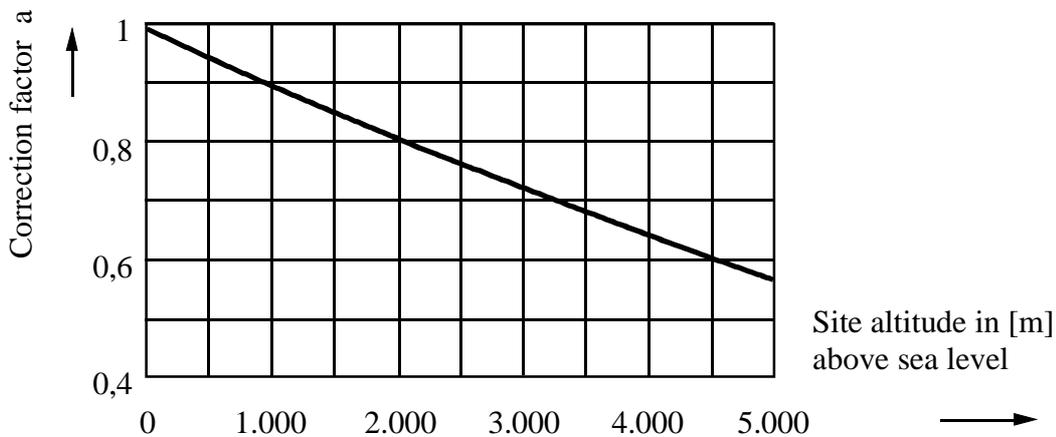
**Figure D-2: Correction factor for the insulating capacity**
