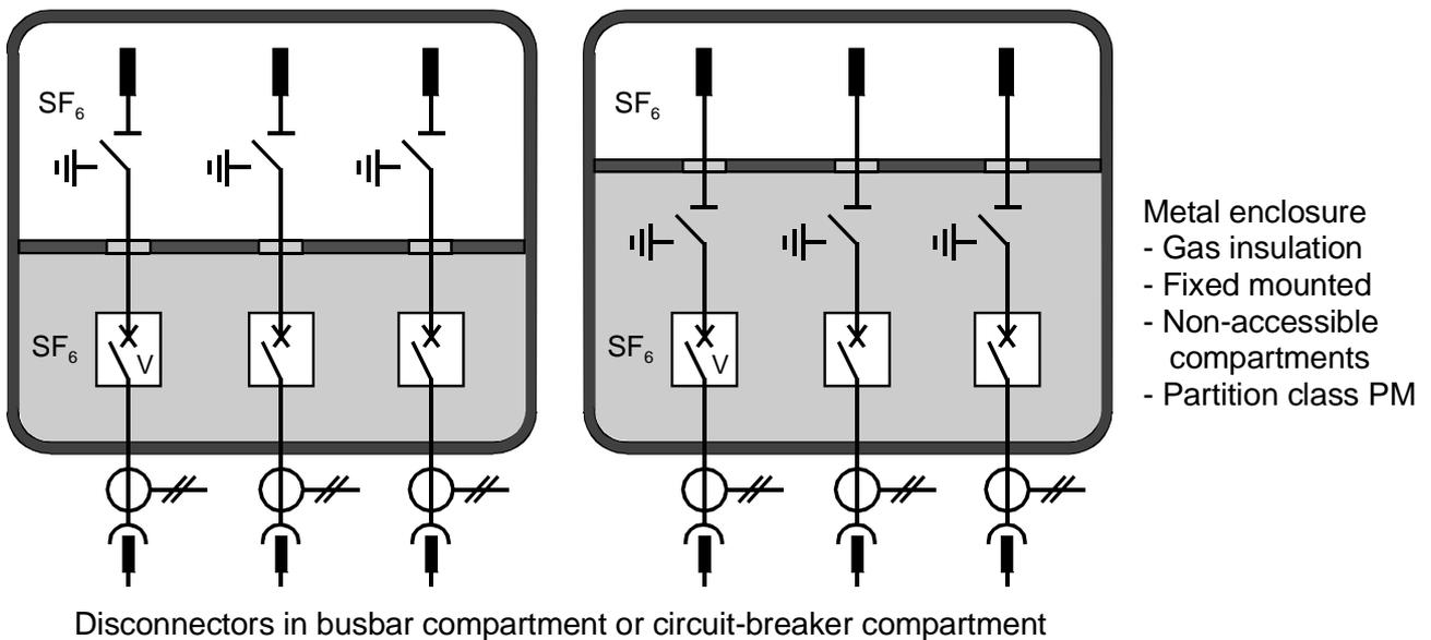
**Figure E-7: GIS design with three-pole encapsulation**
