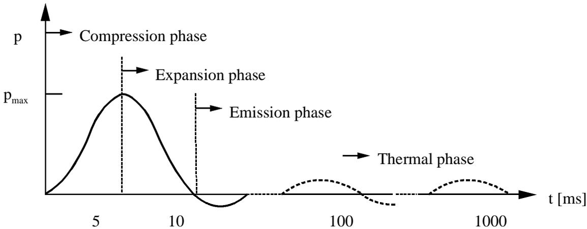
**Figure D-12: Basic pressure characteristic of a fault arc**
