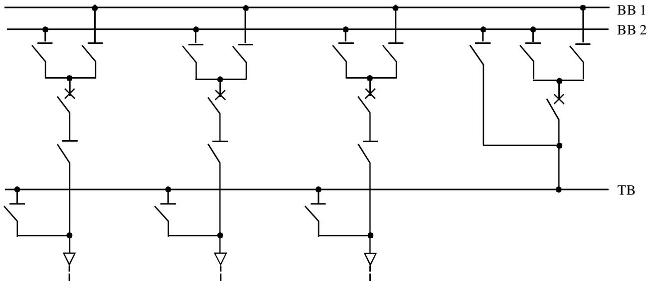
**Figure D-5: Transfer busbar**
