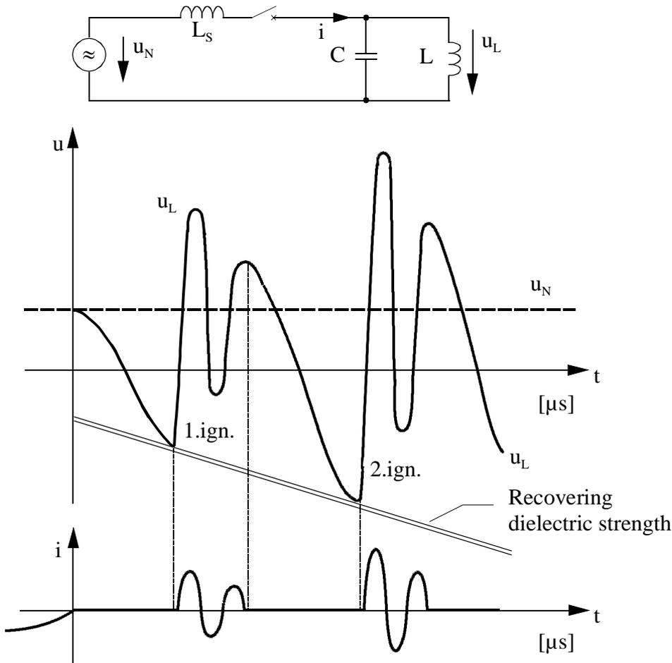
**Figure B-3: Reignitions during inductive switching (principle)**
