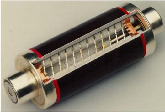
The ceramic body is filled with silica sand as quenching medium. The fusible elements – depending on their rated current, there can be more than one connected in parallel – are wound around a ceramic star. The striker with auxiliary fusible element can be seen in the longitudinal axis.
