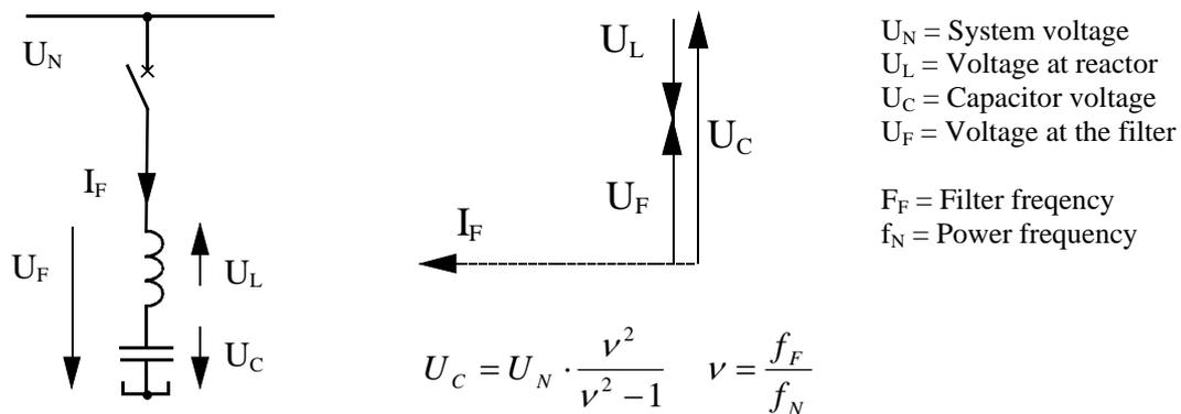
**Figure B-13: Voltages of a filter circuit**
