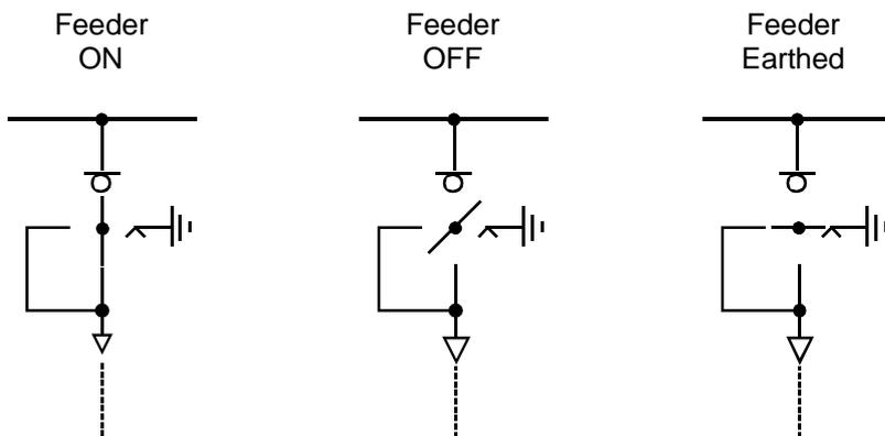
**Figure E-22: Example of a three-position switch**
