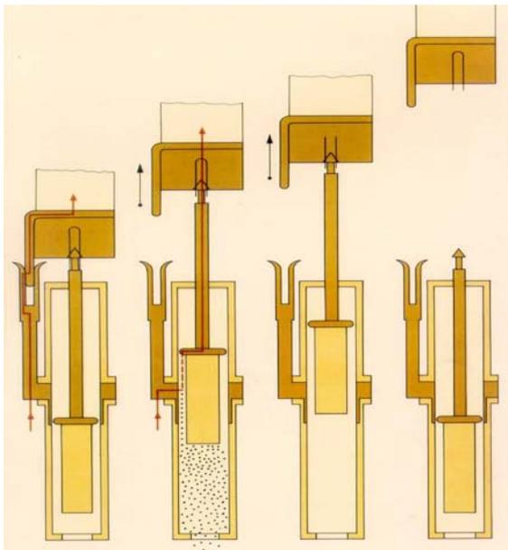
Figure C-10 shows a diagram of the breaking operation with main and quenching contact (Siemens Type 3CF).
