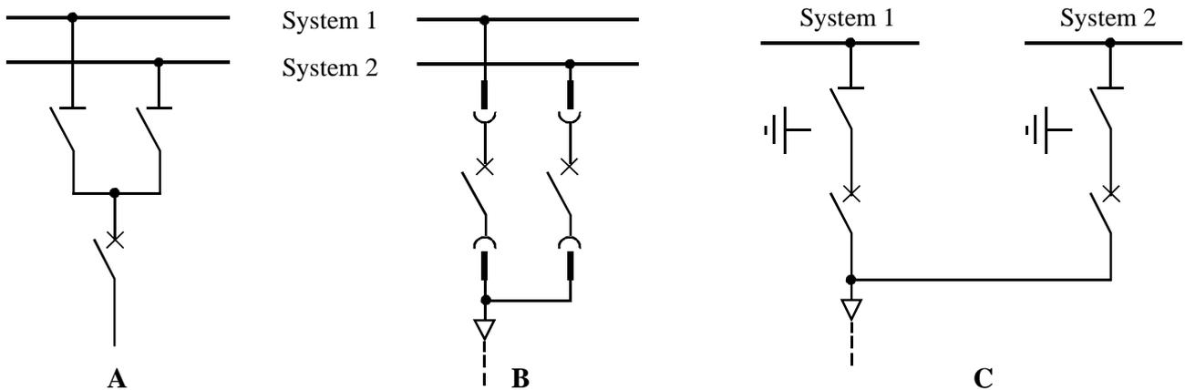
**Figure D-10: Disconnector arrangements in double busbar switchgear**
