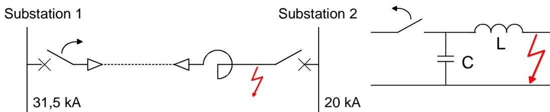
**Figure B-20:** Short-circuit downstream current limiting reactor
