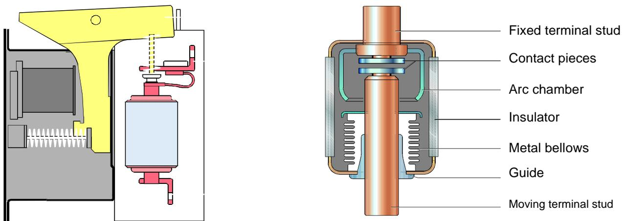
**Figure C-13: Principle of a vacuum contactor and an interrupter**
