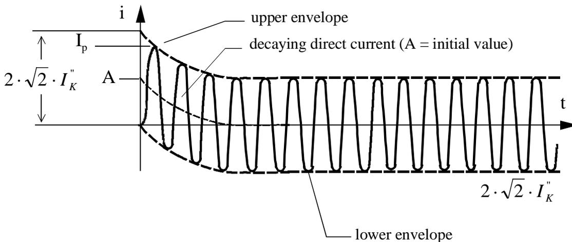
**Figure B-14: Short-circuit remote from generator (short-circuit in the system)**
