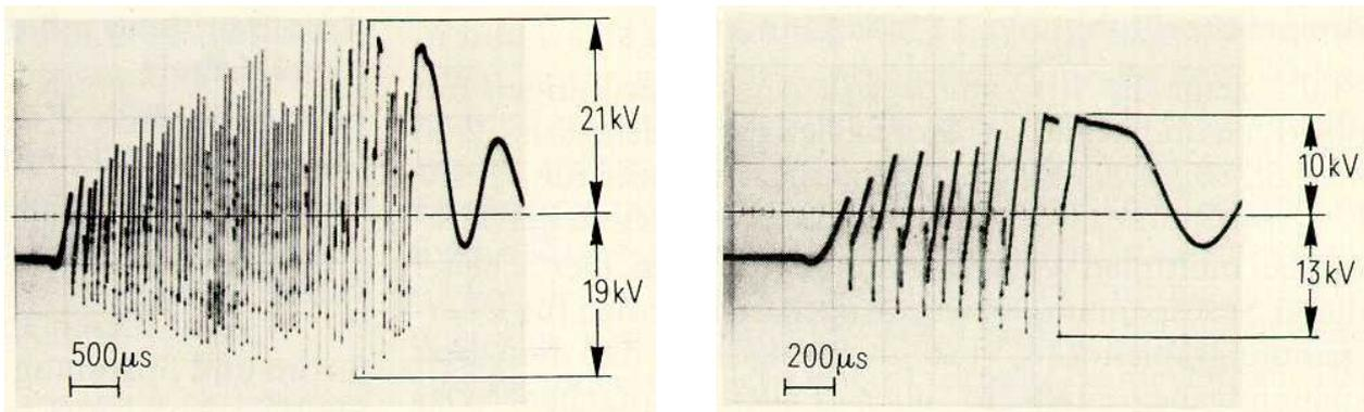
Multiple reignitions in the breaking of a purely inductive 6 kV circuit; without voltage limiting (left) and with voltage limiting (right).
