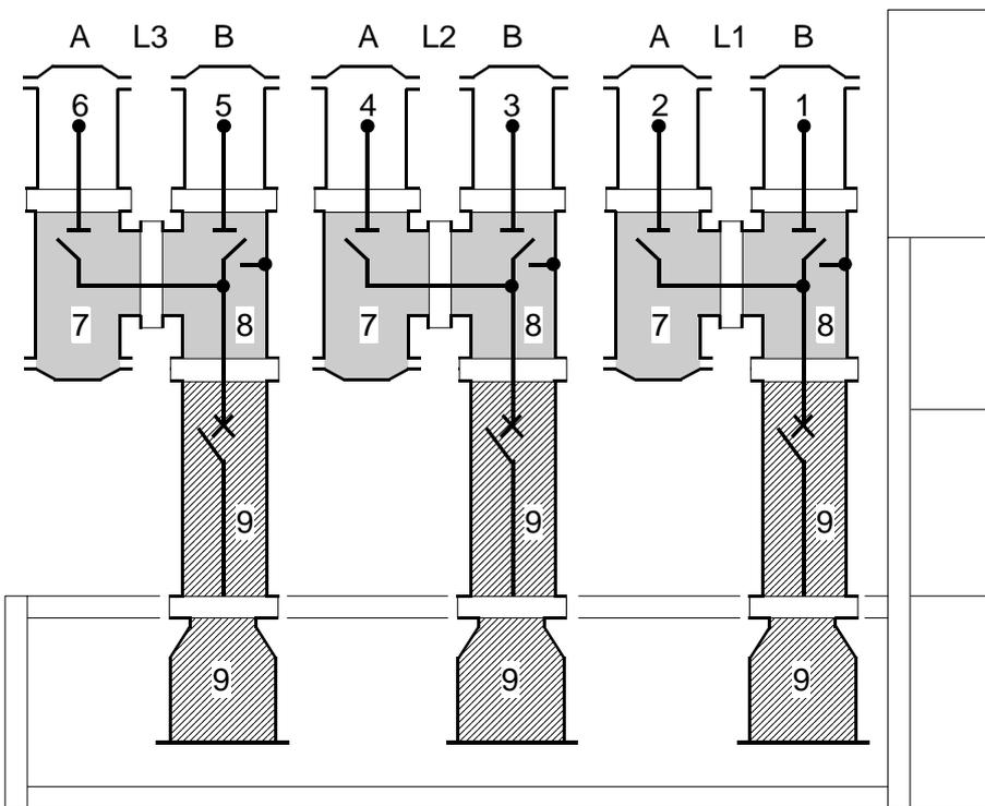
**Figure E-19: Gas compartments of a single-pole encapsulated switchgear longitudinal section (equal numerals = equal gas compartments)**
