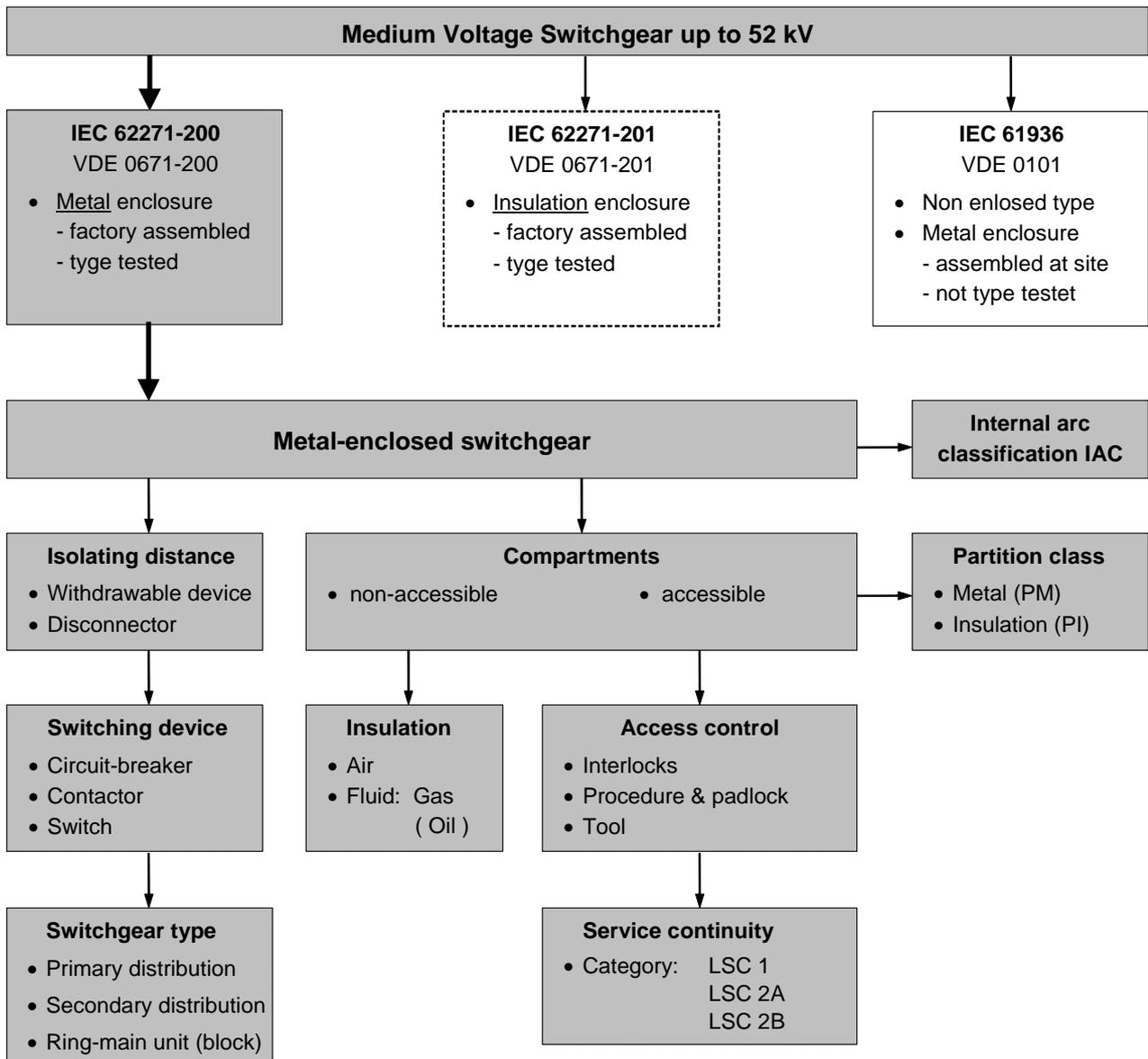
**Figure E-1: Classifications of the switchgear designs**
