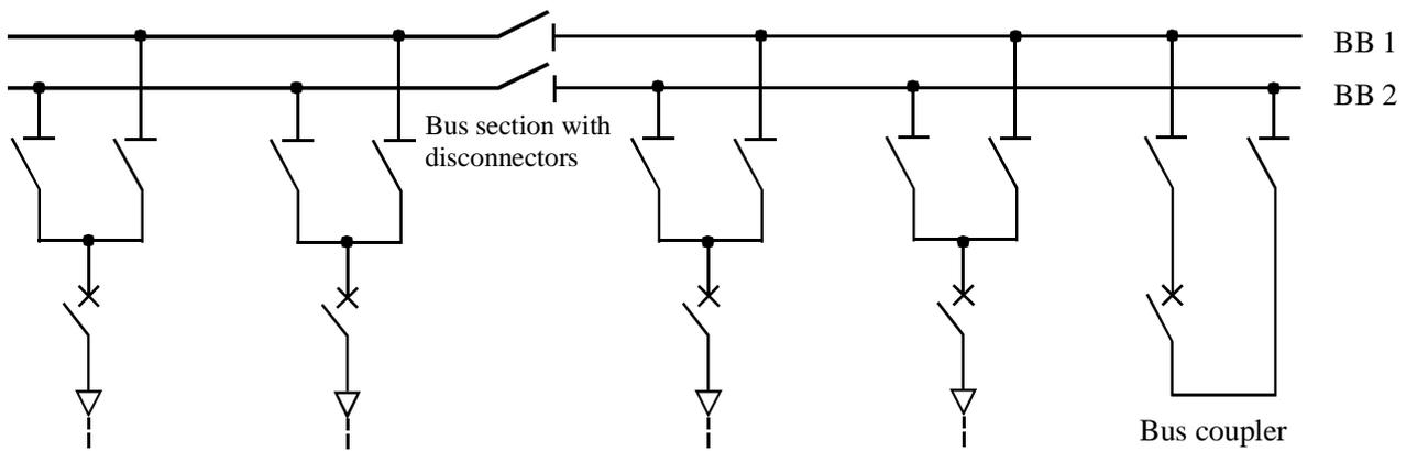
**Figure D-4: Double busbar with a bus section with disconnectors and a bus coupler**
