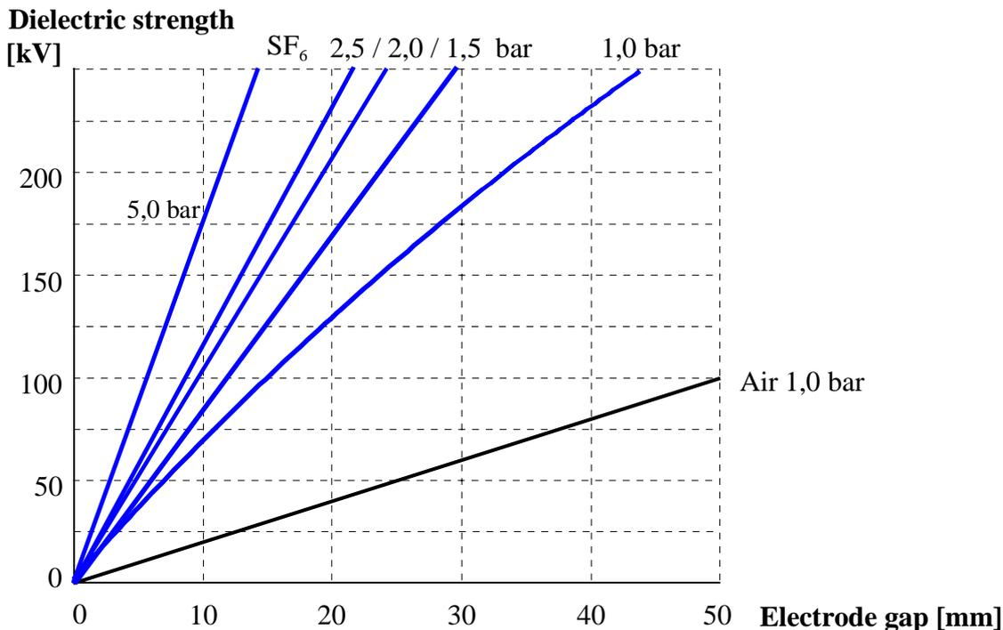
**Figure G-1: Breakdown voltage at 50 Hz in homogeneous fields – air and SF<sub>6</sub>**
