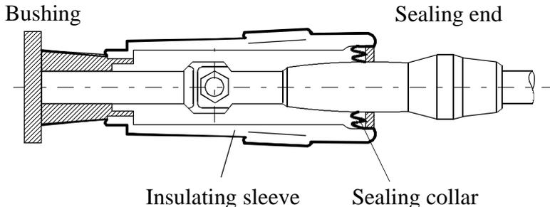
**Figure F-3: Sealing end with insulation sleeve**
