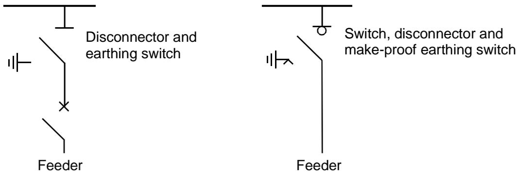
**Figure C-12: Pattern of three-position disconnector or switch**
