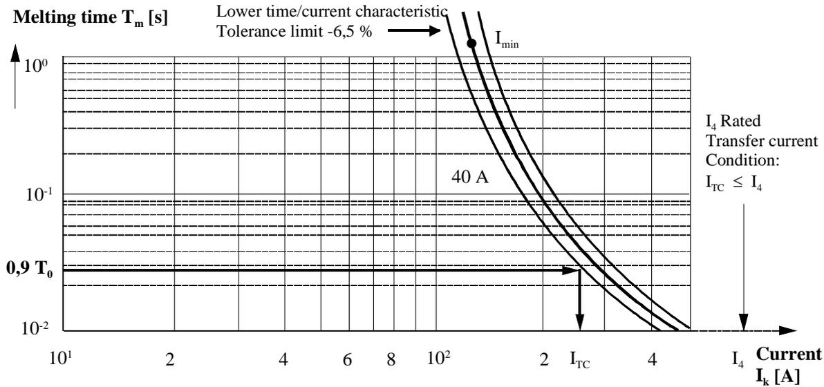
**Figure C-22: Determination of the transfer current from a fuse characteristic**
