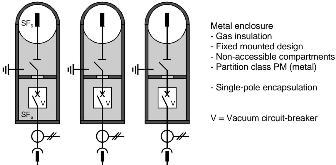
**Figure E-6: GIS design with single-pole encapsulation**
