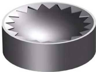
In the event of impermissible internal pressure, the concave membrane bends outwards and is cut open by the sharp metal points.
