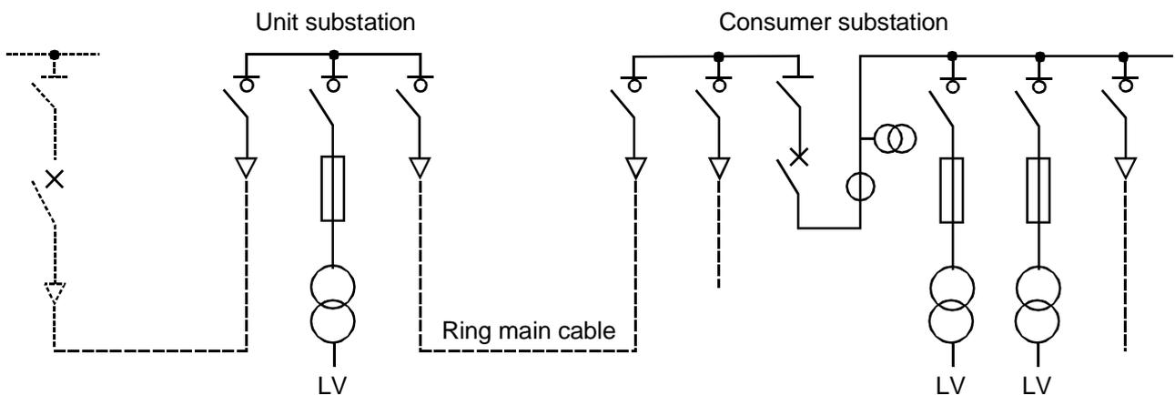
**Figure D-6: Unit and consumer substations in a cable ring**
