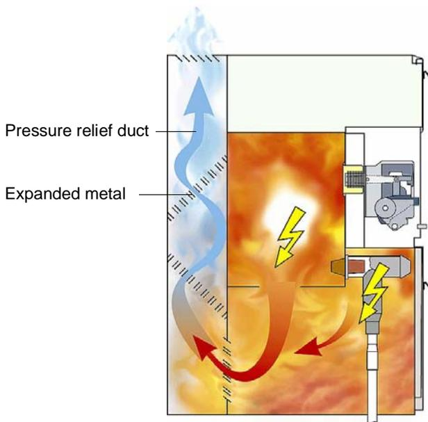
**Figure D-13: Absorbers damp the overpressure in the building**
