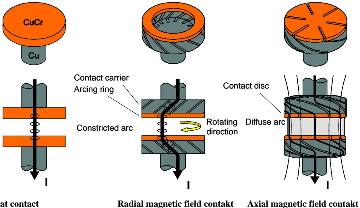
**Figure C-8: Contact types for vacuum circuit-breakers**
