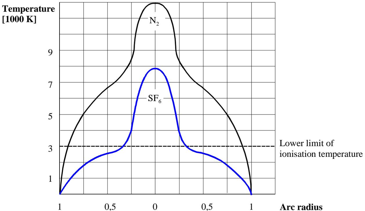
**Figure G-2: Radial temperature distribution within an arc in SF<sub>6</sub> and N<sub>2</sub>**
