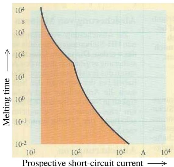
**Figure C-19: Current/time characteristic of a full-range fuse**
