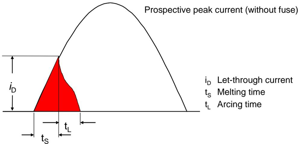
**Figure C-16: Breaking operation of an HRC fuse**
