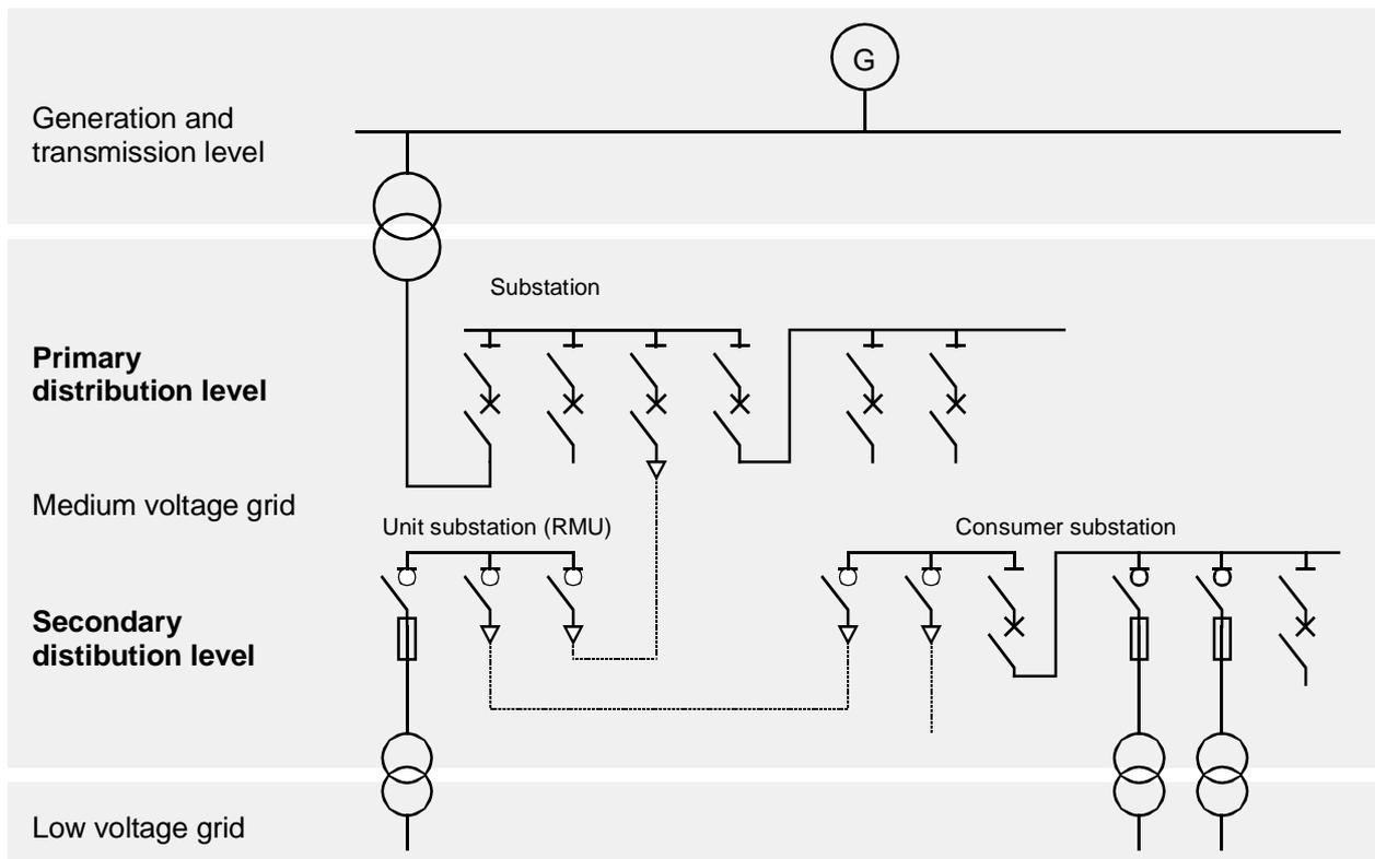
**Figure D-1: Main uses for substations in the distribution network**
