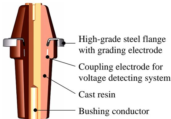
Weldable outer cone bushing (sectional view ) for gas-insulated switchgear
