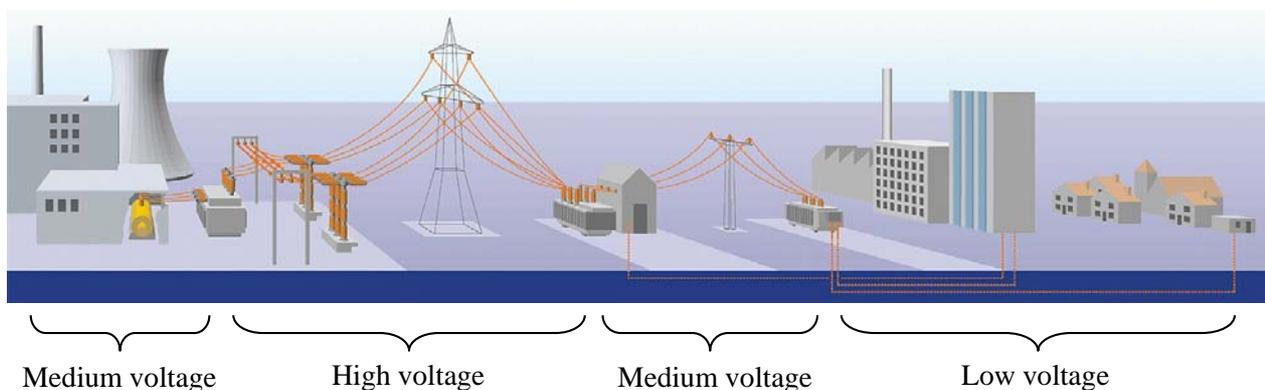
**Figure A-2: Voltage levels from the generating plant to the consumer**
