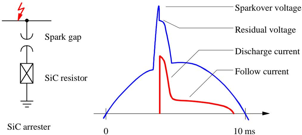
Figure C-27: Structure and mode of operation of SiC-arresters with spark gaps
