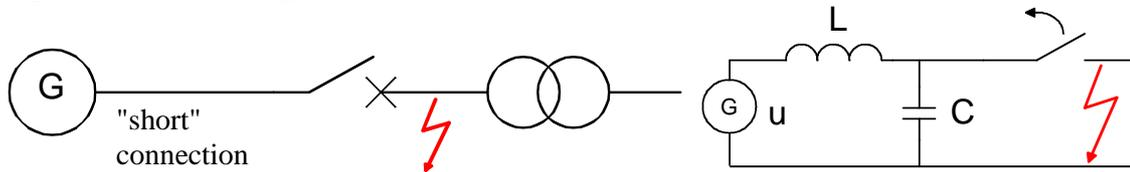
**Figure B-19:** Short-circuit downstream generator
