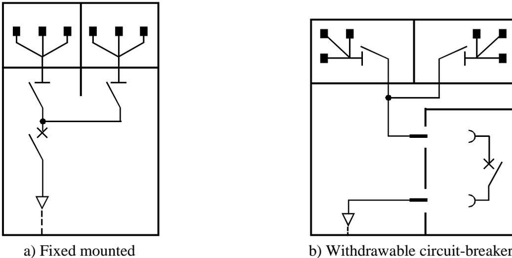
**Figure D-7: Double busbar switchgear, fixed mounted disconnectors**
