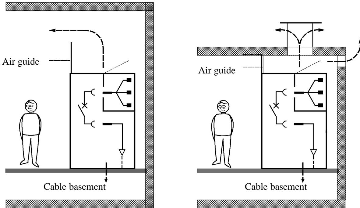
**Figure D-14: Pressure relief (example) for high and low buildings**
