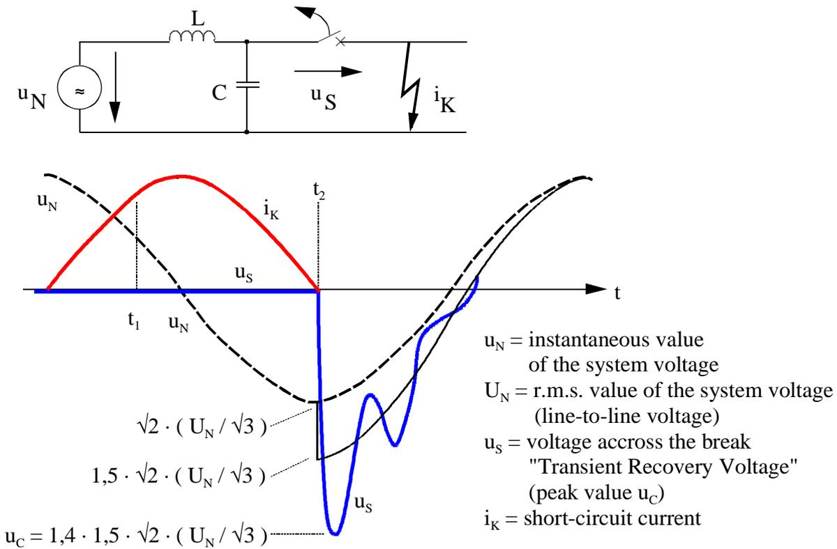
**Figure B-17: Transient recovery voltage after short-circuit in the system**
