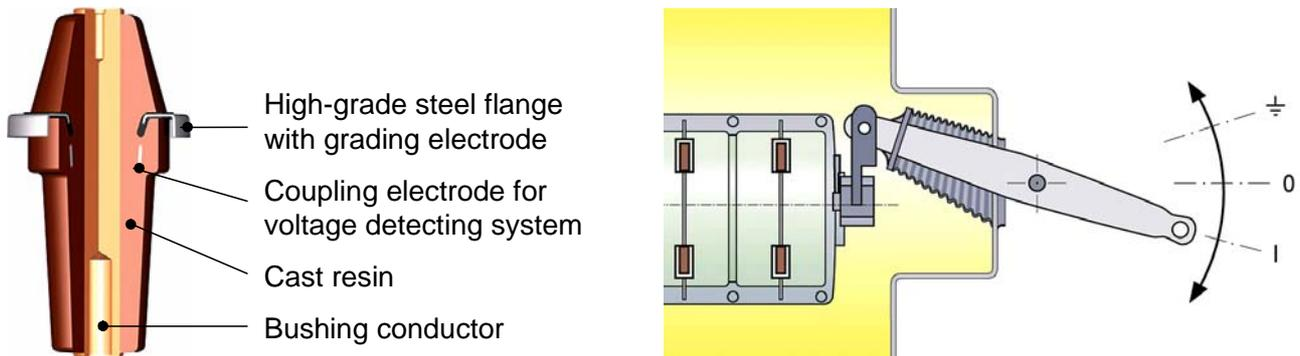
**Figure E-13: Gas-tight bushing for conductor and gas-tight penetration for drive lever**
