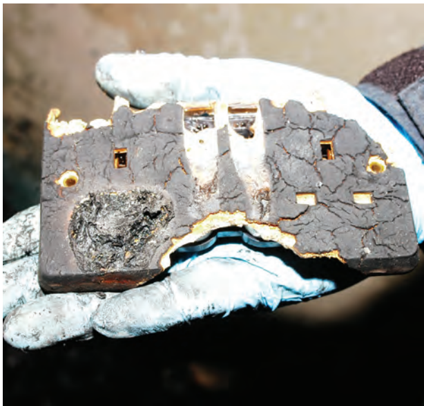
The effect of fire on a socket-outlet (Photo courtesy of Greater Manchester Fire & Rescue Service)
