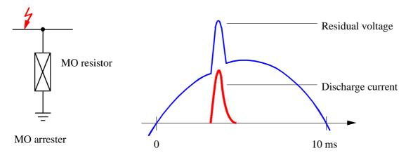
Figure C-28: Structure and mode of operation of MO-arresters
