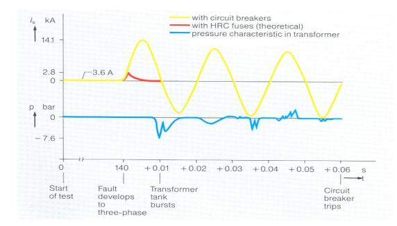
Figure C-25: Fault development in a distribution transformer
