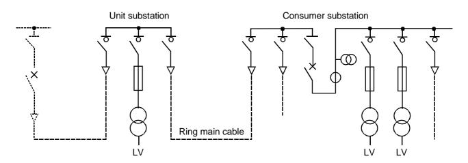
Figure D-6: Unit and consumer substations in a cable ring
