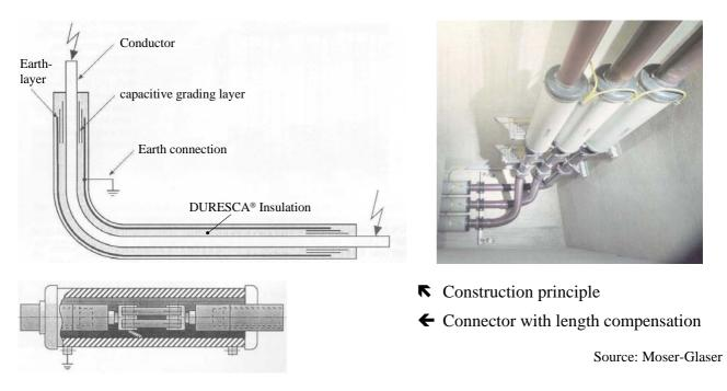
Figure F-1: Solid insulated bar
