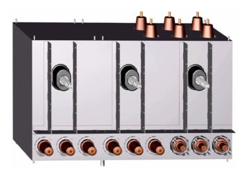
The illustration shows a load switch block (RMU) for two ring cables and a transformer feeder with HRC fuse. The welded conductor bushings for fitting the fuse boxes can be seen at the top; below are the conical bushings of various sizes for the network cables (left and center) and the cable to the transformer. The middle of the vessel features the welded bellows for the moving mechanism parts.
