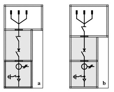
Figure E-24: Variants of compartmented "fixed mounted" designs
