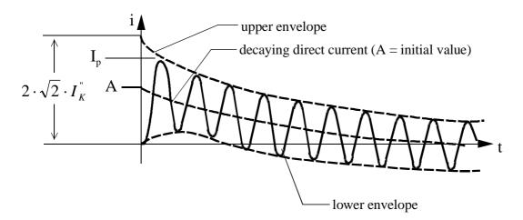
Figure B-16: Short-circuit close to generator woth missing current zeros
