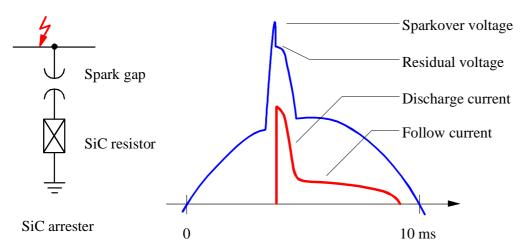
Figure C-27: Structure and mode of operation of SiC-arresters with spark gaps
