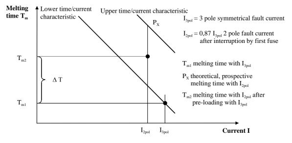
Figure C-23: Melting time of fuse in the region of the transfer current
