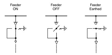
Figure E-22: Example of a three-position switch
