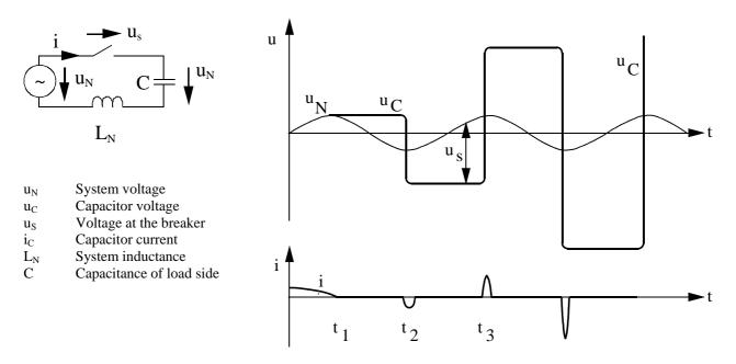
Figure B-11: Restrikes during capacitive switching
