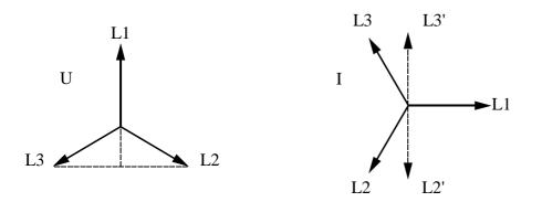
Figure B-18: Vector diagram of a short-circuit in the system
