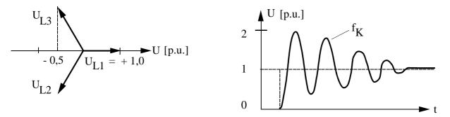
Figure B-8: Voltages at time t<sub>1</sub> and voltage trace in first pole to close
