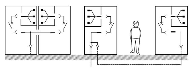
Figure D-8: Back-to-back and face-to-face arrangement
