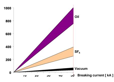
Figure C-9: Arc energy in different quenching media in the comparison
