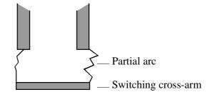
Some of these disadvantages were overcome by the introduction of arc chambers under the oil. The switching characteristics of these designs correspond approximately to those of minimum-oil circuit-breakers with a current-dependent arcquenching effect.
