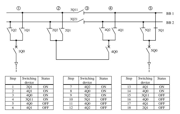
Figure D-9: Example for a busbar transfer
