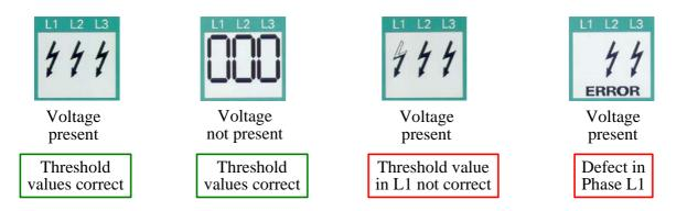
Figure F-13: Indication data with a LC-Display
