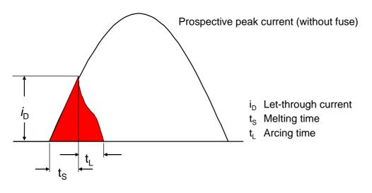
Figure C-16: Breaking operation of an HRC fuse
