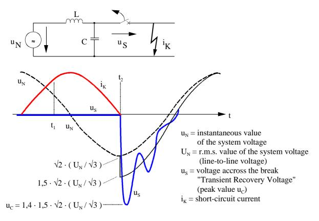
Figure B-17: Transient recovery voltage after short-circuit in the system
