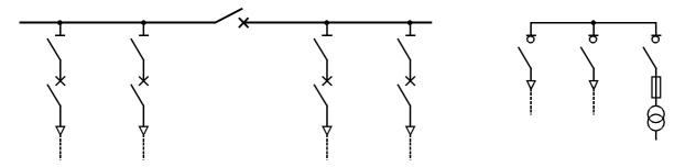
**Figure D-3:** Single busbar with sectionalizer (left) and in a unit substation (right)
