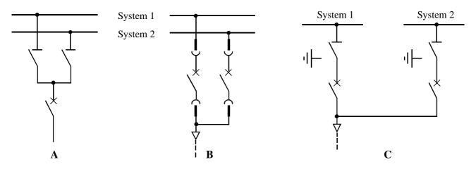
Figure D-10: Disconnector arrangements in double busbar switchgear
