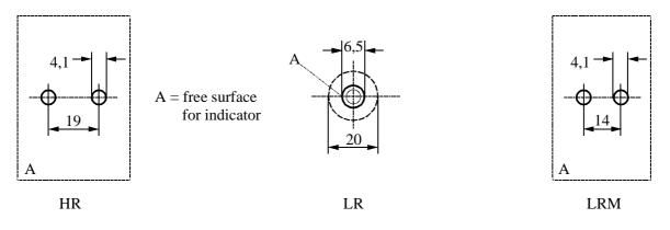
Figure F-12: Interfaces of separable VDS
