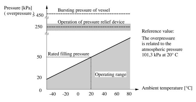
Figure E-11: Pressure range of a representative GIS (example)
