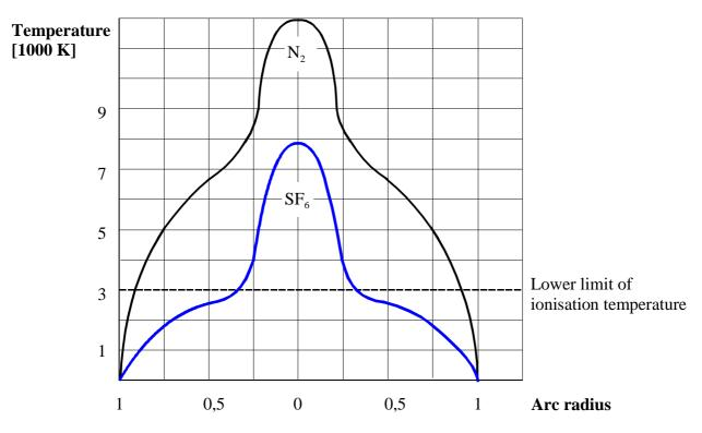
Figure G-2: Radial temperature distribution within an arc in SF<sub>6</sub> and N<sub>2</sub>
