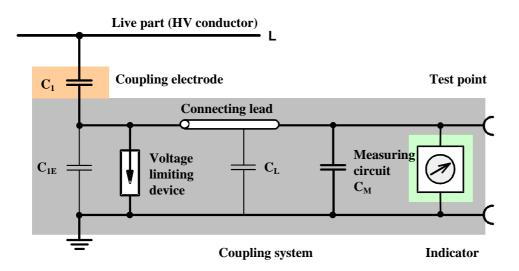
Figure F-9: Scheme of an integrated voltage detecting system
