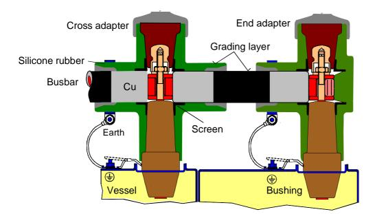
Figure E-10: Pluggable busbar with silicone rubber insulation
