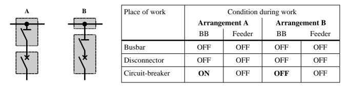
Figure E-16: Influence of location of disconnector on the service continuity of single busbar
