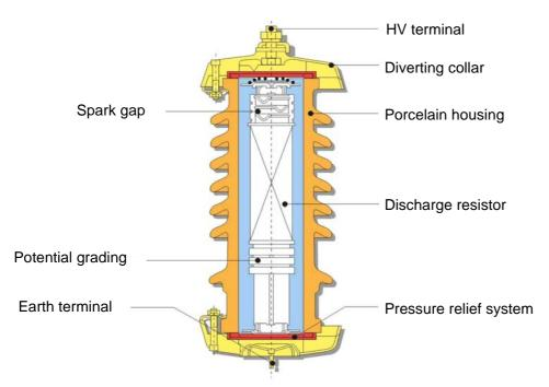
Figure C-26: Surge arrester (example Siemens 3EG type)
