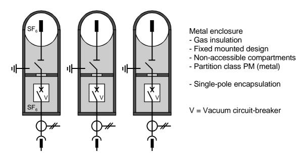
Figure E-6: GIS design with single-pole encapsulation
