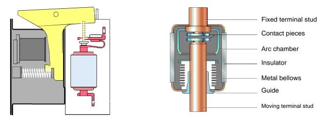
Figure C-13: Principle of a vacuum contactor and an interrupter
