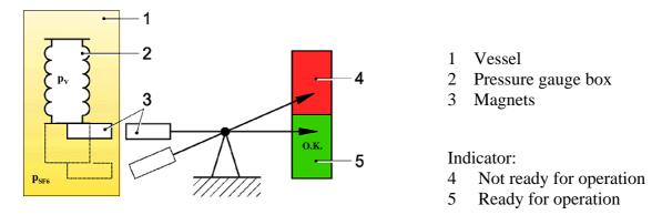
Figure E-15: Gas pressure monitoring, example of a qualitative indication
