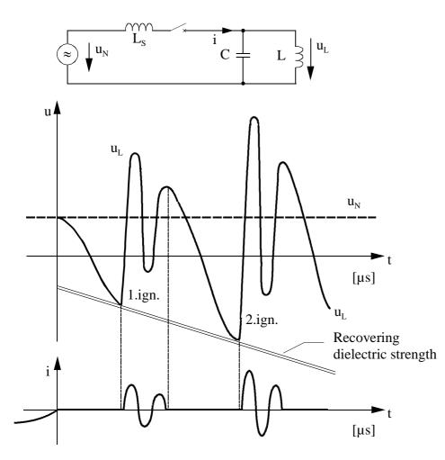
Figure B-3: Reignitions during inductive switching (principle)
