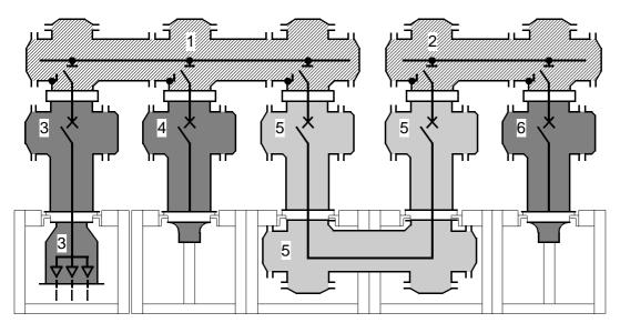
**Figure E-18:** Gas compartments of a single-pole encapsulated switchgear cross-section of double busbar (equal numerals = equal gas compartments)
