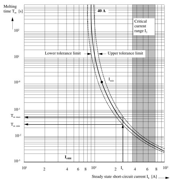
Figure C-18: Current/time characteristic of an HRC fuse
