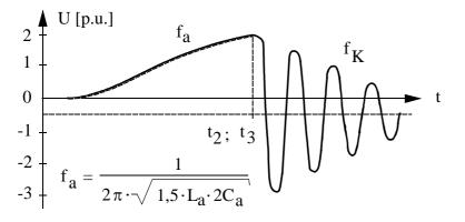
Figure B-10: Voltage trace in last poles to close
