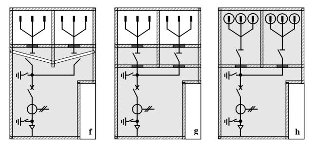
Figure E-26: Cubicle design double busbar switchgear
