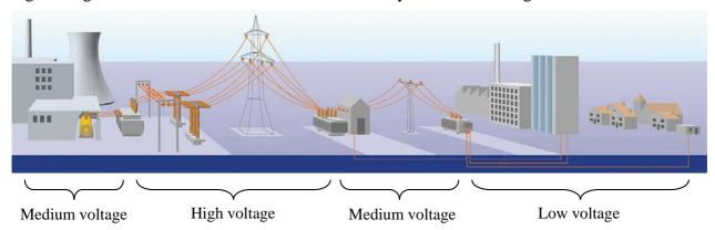
Figure A-2: Voltage levels from the generating plant to the consumer
