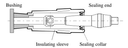
Figure F-3: Sealing end with insulation sleeve
