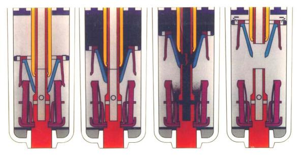
Figure C-4: Arc-quenching principle of an SF<sub>6</sub>-puffer type circuit-breaker
