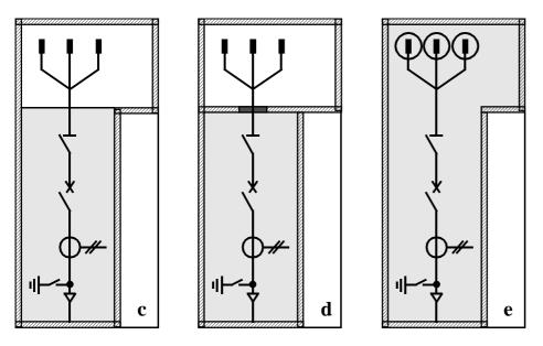
Figure E-25: Variants of "fixed mounted"cubicle designs
