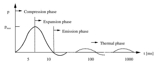
Figure D-12: Basic pressure characteristic of a fault arc
