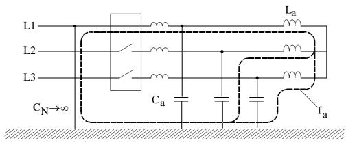
Figure B-9: Oscillations in last poles to close before contacts touch
