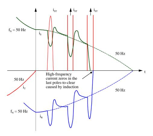
Figure B-6: Virtual (induced) current chopping in the phases S and R
