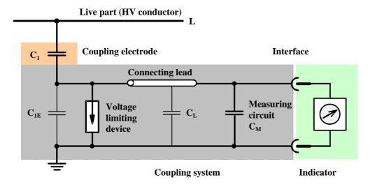
Figure F-8: Scheme of a separable voltage detecting system
