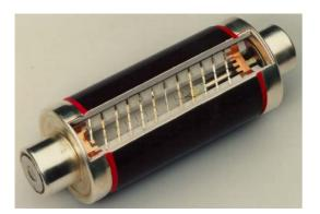
The ceramic body is filled with silica sand as quenching medium. The fusible elements – depending on their rated current, there can be nmore than one connected in parallel – are wound around a ceramic star. The striker with auxiliary fusible element can be seen in the longitudinal axis.
