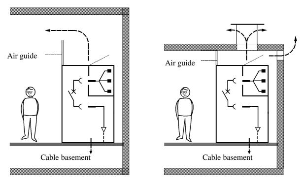
Figure D-14: Pressure relief (example) for high and low buildings
