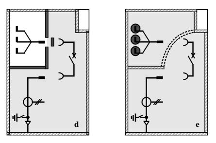
Figure E-4: Cubicle design with withdrawable or truck-type switching device
