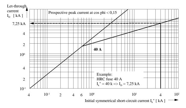
Figure C-17: Cut-off characteristic of an HRC fuse
