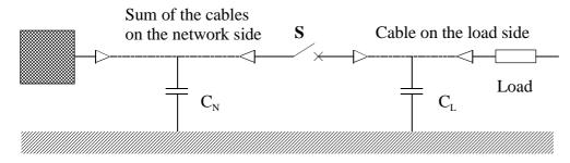
Figure B-24: Network conditions or earth fault before and after a breaker
