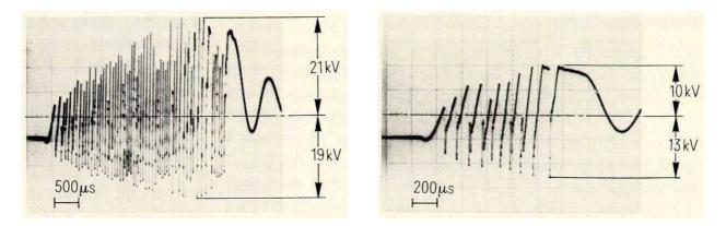
Multiple reignitions in the breaking of a purely inductive 6 kV circuit; without voltage limiting (left) and with voltage limiting (right).
