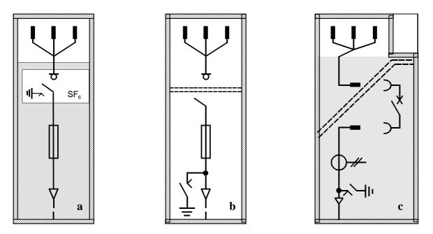
Figure E-20: Variants of feeder-type (extensible) design
