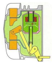
Figure C-5: Example of an self-extinguishing SF<sub>6</sub> circuit-breaker
