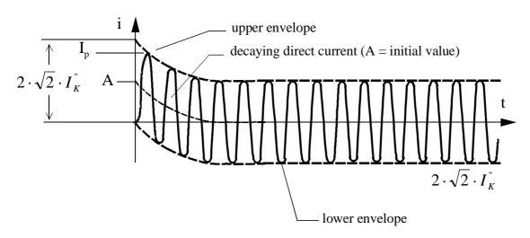
Figure B-14: Short-circuit remote from generator (short-circuit in the system)
