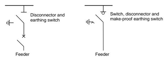
Figure C-12: Pattern of three-position disconnector or switch
