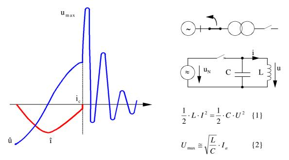
**Figure B-2: Current chopping during inductive switching**
