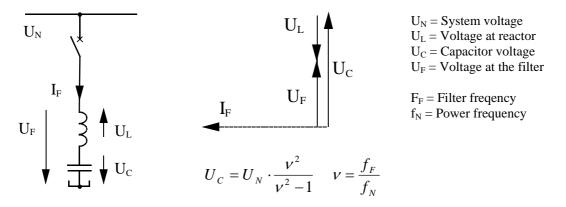
Figure B-13: Voltages of a filter circuit
