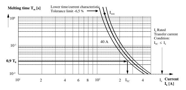
Figure C-22: Determination of the transfer current from a fuse characteristic
