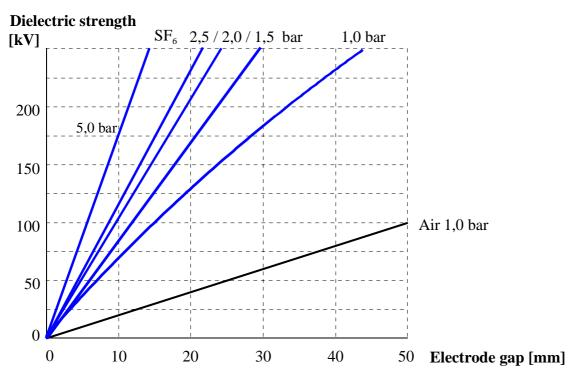
Figure G-1: Breakdown voltage at 50 Hz in homogeneous fields – air and SF<sub>6</sub>
