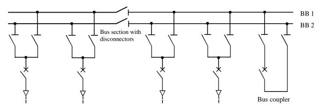
Figure D-4: Double busbar with a bus section with disconnectors and a bus coupler
