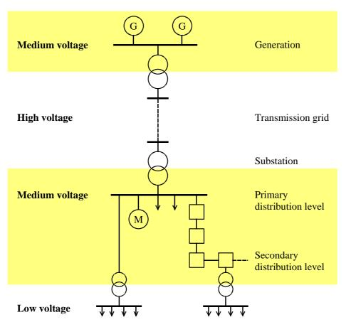
Figure A-3: Medium voltage in an electricity supply network
