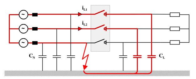
Route of the capacitive load current, e.g. in the healthy phase L2, that must be switched off by the breaker.
