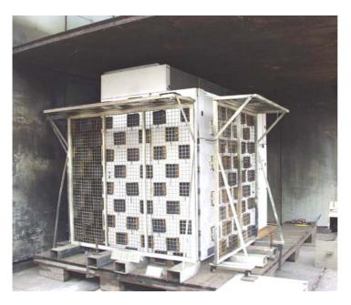
Horizontal and vertical material indicators arranged in a chessboard pattern show whether – during the arc- dangerous hot gases escape from the enclosure.
