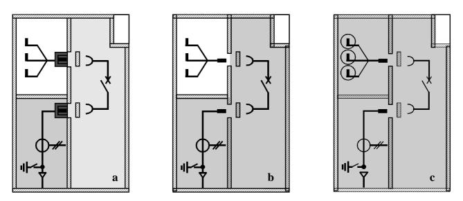
Figure E-3: Withdrawable or truck-type design with "compartmentalization"
