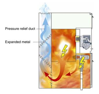
Figure D-13: Absorbers damp the overpressure in the building
