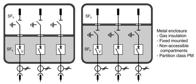
Disconnectors in busbar compartment or circuit-breaker compartment
