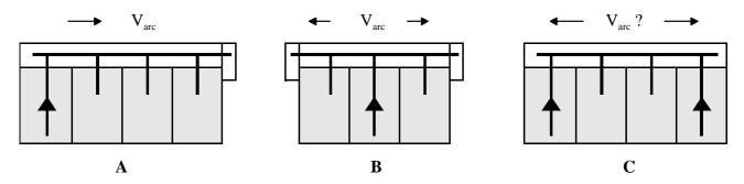
Figure E-5: Direction of fault arc travel for various locations of incomer
