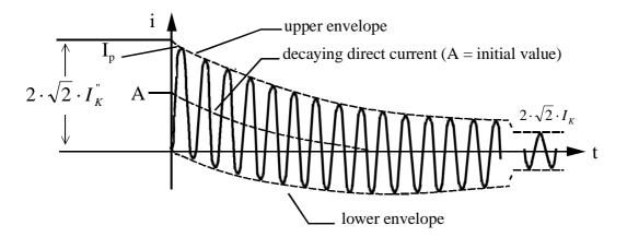
Figure B-15: Short-circuit close to generator
