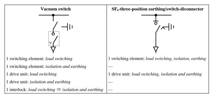
Figure E-23: Consequences of the type of switching device in GIS secondary switchgear
