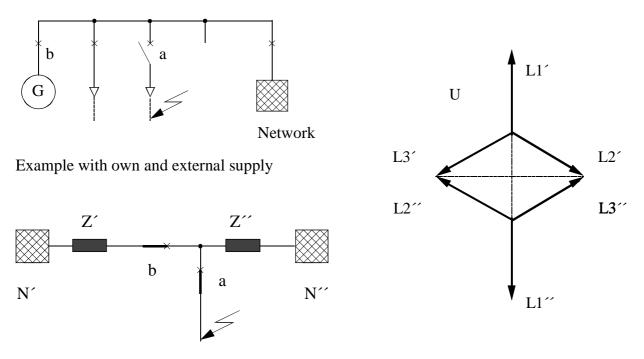
Figure B-23: Switching off under out-of-phase condition
