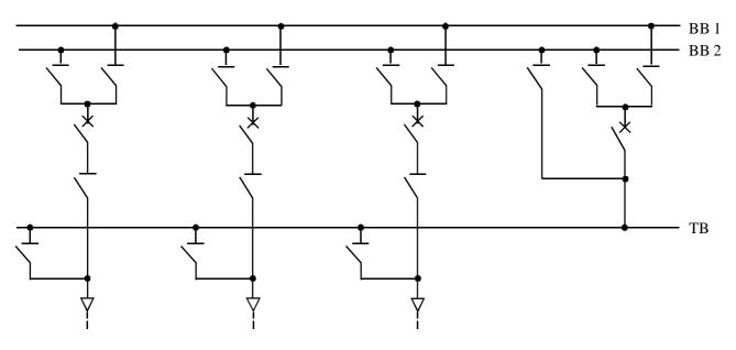
Figure D-5: Transfer busbar
