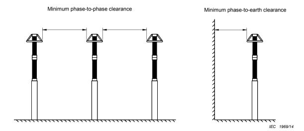
Figure F.1 – Typical three-phase arrester installation
