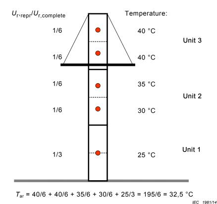
Figure J.1 – Determination of average temperature in case of arrester units of same rated voltages
