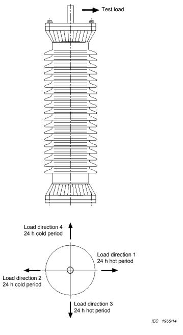
Figure 12 – Example of the test arrangement for the thermomechanical test and direction of the cantilever load
