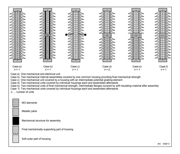
Figure 5 - Examples of arrester units
