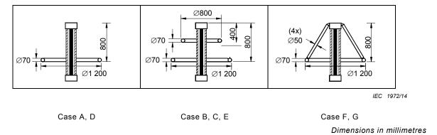
Figure F.3b - Different representations of the grading ring
