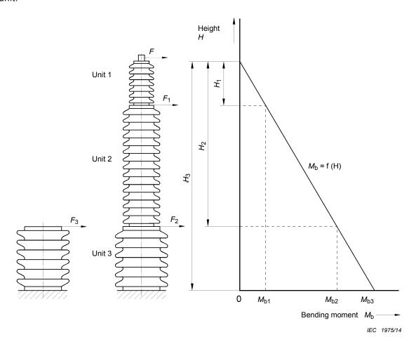
Figure G.1 - Bending moment - multi-unit surge arrester
