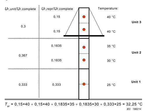
Figure J.2 – Determination of average temperature in case of arrester units of different rated voltages
