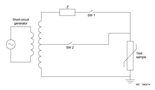
NOTE SW 1 is closed and SW 2 is opened to apply pre-failing level of current (maximum of 30 A, limited by impedance Z). After a maximum of 2 s, SW 2 is closed to cause the specified short-circuit current to flow through the test sample.
