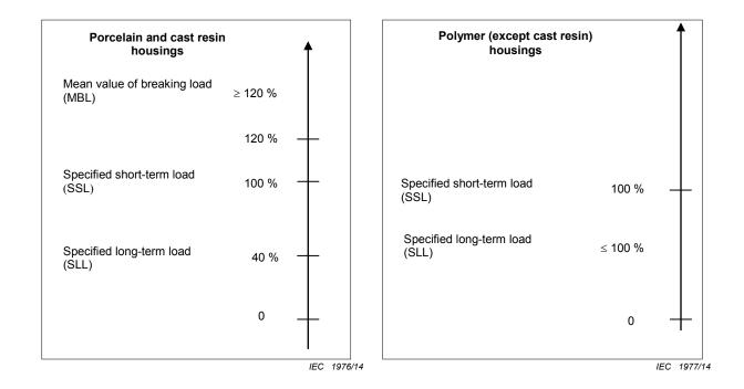
Figure G.2 – Definition of mechanical loads
